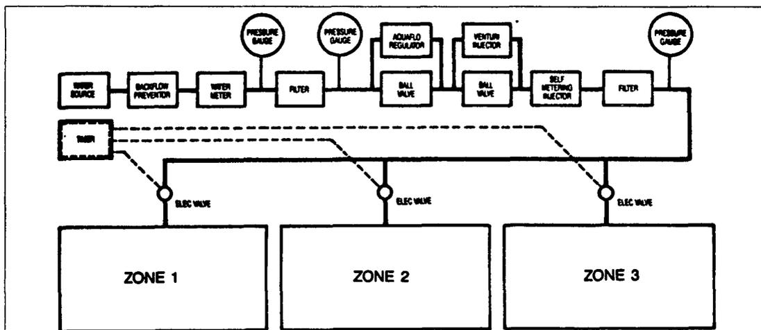
Figure 9. Component Layout from Water Source to Irrigation Zones (*Installation, Operation and Maintenance Instructions for Aquapore Subsurface Irrigation Systems*, 1989, p. 3-4).
