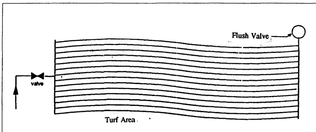
Figure 6. Ram Tubing Layout for Turf (Netafim Irrigation Equipment & Drip Systems, 1986, p. 8).
