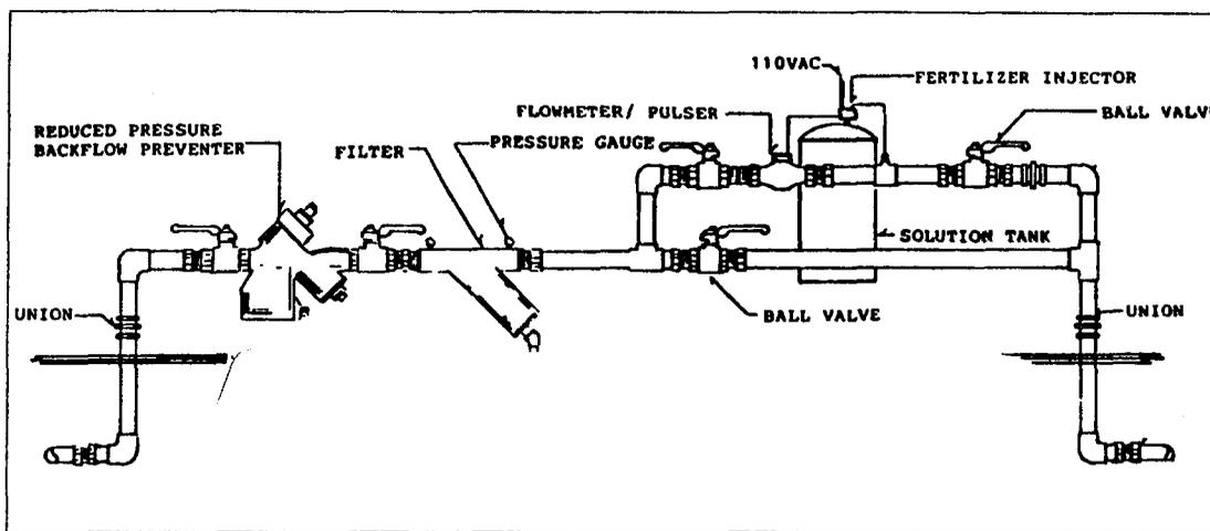
Figure 11. Valve Manifold Assembly (Aquapore-Installation Specifications and Construction Details, 1989, p. 7).
