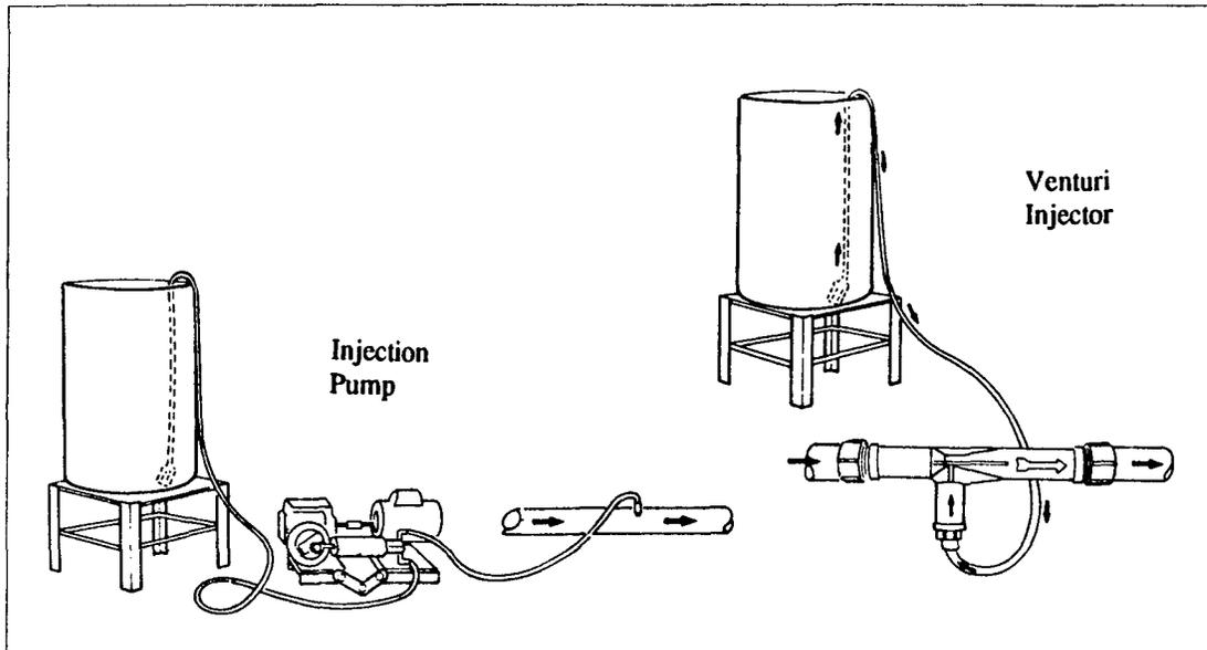
Figure 3. Chemical Injection Devices (Boswell, 1986, pp. 5-11).
