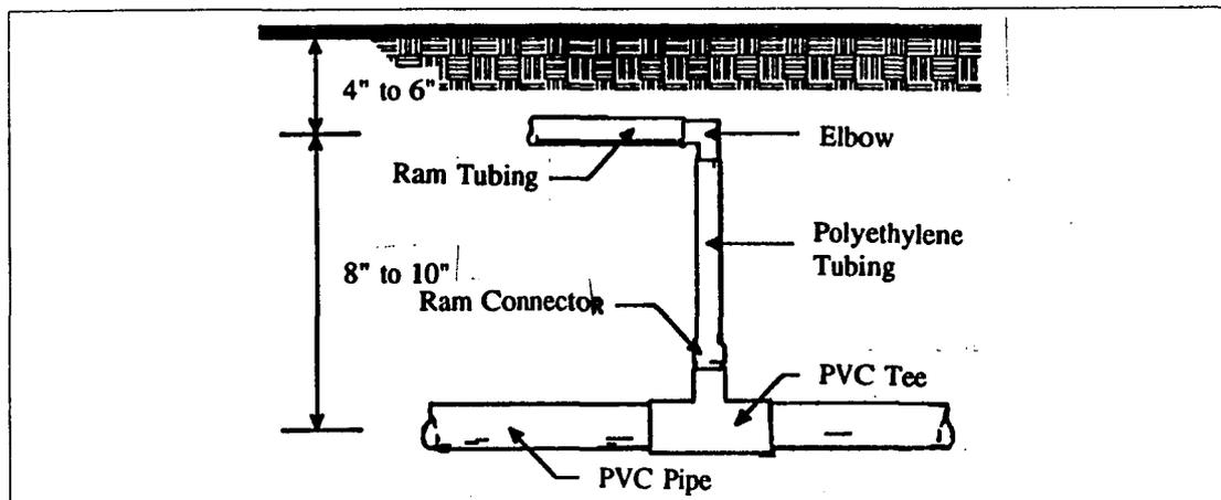
Figure 5. Ram Tubing Depth and Connection to PVC Lateral (Netafim Irrigation Equipment & Drip Systems, 1986, p. 6).
