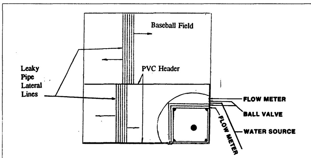
Figure 8. Baseball Field Layout (*Leaky Pipe Subsurface Dispersal Systems*, 1990, p. 34).
