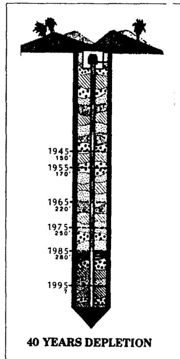
Figure 1. Effect of Water Mining on the Groundwater Table (Johnson, 1985, p. 5).
