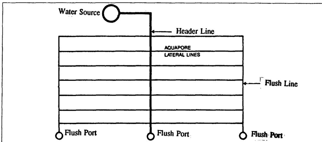
Figure 10. Emitter Tubing Layout Showing Lateral and Flush Valves (Installation, Operation and Maintenance Instructions for Aquapore Subsurface Irrigation Systems, 1989, p. 6-2).
