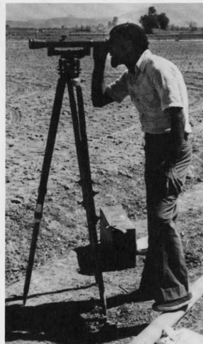
At the research farm that the University of Arizona helped develop in Yemen, assistant engineer Madhu S. Acharya of India surveys a field for leveling.
