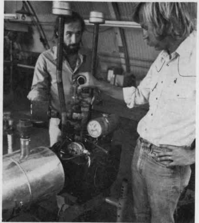
Dr. Williams (left) and student Ed Jorgensen discuss the routing of fuel gas into a pump engine. The hydrogen and carbon monoxide gas is produced by a gasifier and cleaned in the electrostatic precipitator at left.
