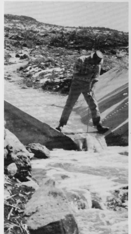
A Forest Service researcher collects a sediment sample at a streamflow-measuring flume. The stream is in an area of pinyon-juniper forest treated to test effects of partial clearing on streamflow. (Photo by Malchus Baker Jr., U.S. Forest Service.)
