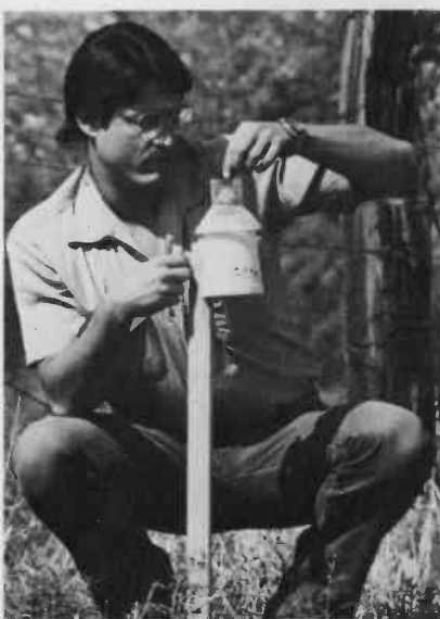
Top: Monitoring traps for boll weevils contain two chips impregnated with the weevils' pheromone, a sex scent that attracts them, plus one chip impregnated with insecticide.
