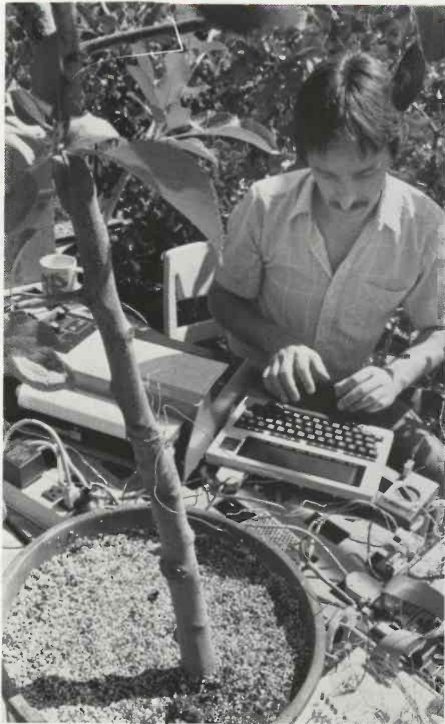
(opposite) Agricultural engineering graduate student Reinaldo Gomide installs an electronic probe into an apple tree. (left) Linked to a computer, the probe measures transpiration by monitoring the sap flow. Knowing the transpiration and water consumption rates will help growers schedule irrigations.
