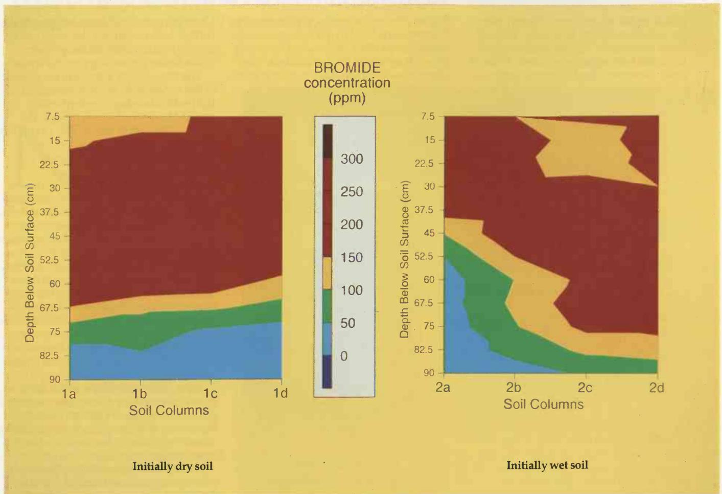
Example of two sites of measured chemical penetration demonstrates patterns of herbicide leaching through wet and dry soils. (Computer artwork by Jon Chernicky)
