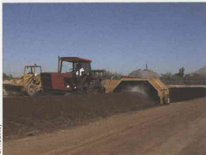
As a part of the composting process, this tractor attachment turns, waters and aerates the manure pile.
