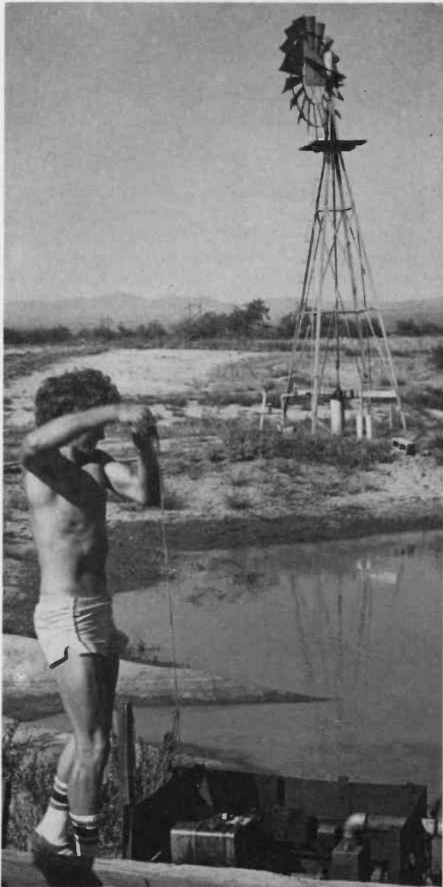
**UA worker John Chamberlain yanks cord to start the diesel pump at the Page Ranch near Oracle. Engineers plan to install a solar pump on the site to compare its performance to the diesel and wind pumps already there.**
