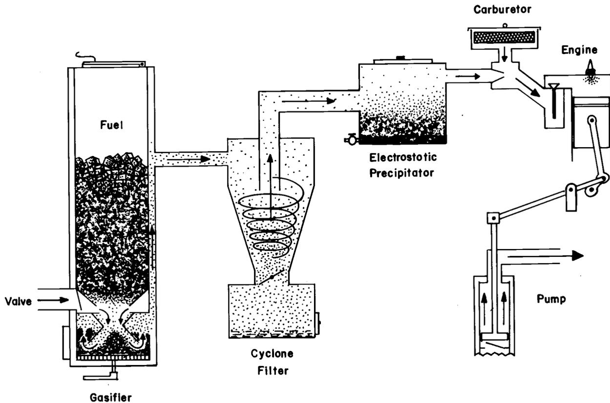
**PRODUCER GASIFIER TO FUEL PUMP ENGINE**—Straw or other fuel is partially oxidized in the gasifier. The valve lets in only enough air for combustion to continue, but not enough for complete oxidation. The reaction produces flammable hydrogen and carbon monoxide gases, which are cleaned in the filter and precipitator, then burned in the internal-combustion engine that drives the pump.
