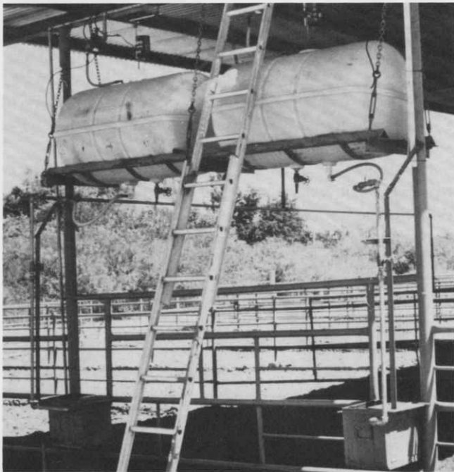
Matching tanks to hold fresh water and salty water were installed for test measurements at the UA dairy farm in Tucson.
