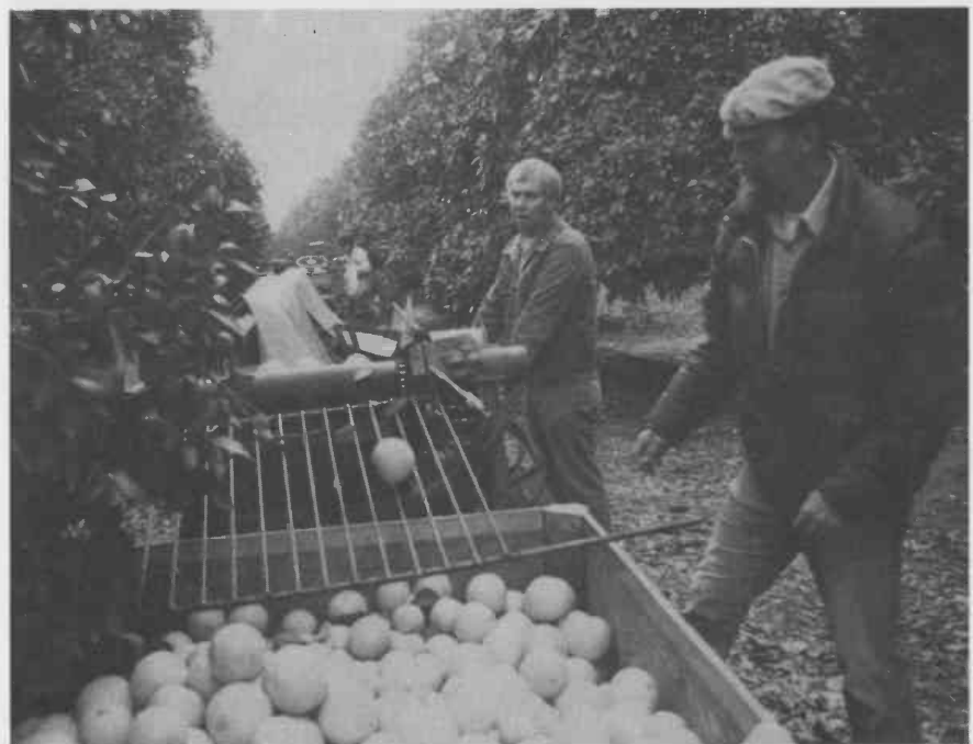
UA citrus farm coordinator Dean Bacon (right) and agricultural engineer Dr. Joe Gentry operate the conveyer system that rolls grapefruit over a grid and into the shipping box.
