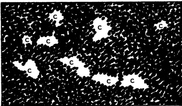
Figure 1. Simplified Model of Paste Structure (Modified after Powers, 1958)
