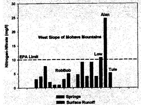
Figure 7. Nitrogen-nitrate of spring concentrations from spring water and from emerging precipitation subflow around the Lake Havasu area.
