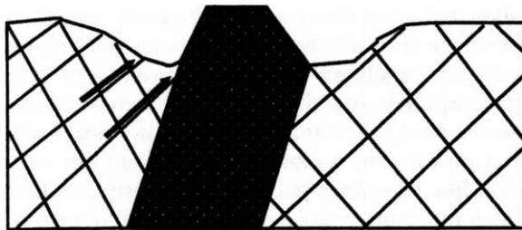
(c) Dike Barrier in Fractured Rock
