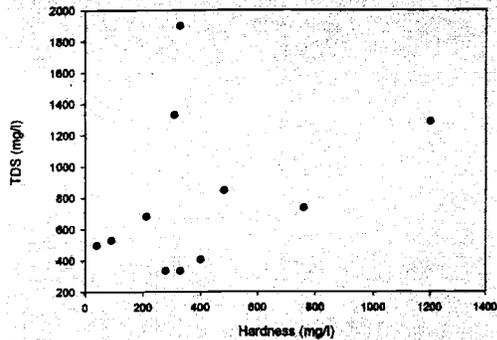
Figure 6. Total dissolved solids vs hardness waters indicate two types of water: calcium cation rich and water containing a greater amount of anions and/or other cations.
