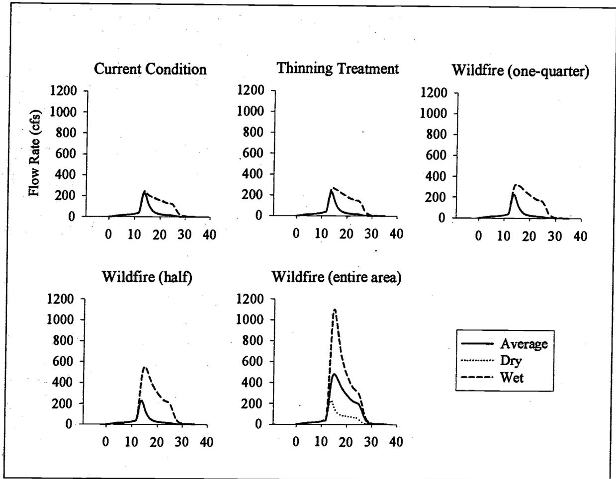
Figure 6. Hydrographs from a 5 yr storm following a wildfire that burned the entire watershed, producing significant flows of about 1100 cfs under wet antecedent soil moisture conditions (AMC) while storms after intensely thinned forest and following fires of lesser extent under all AMC types produce smaller peak discharges of less than 600 cfs.
