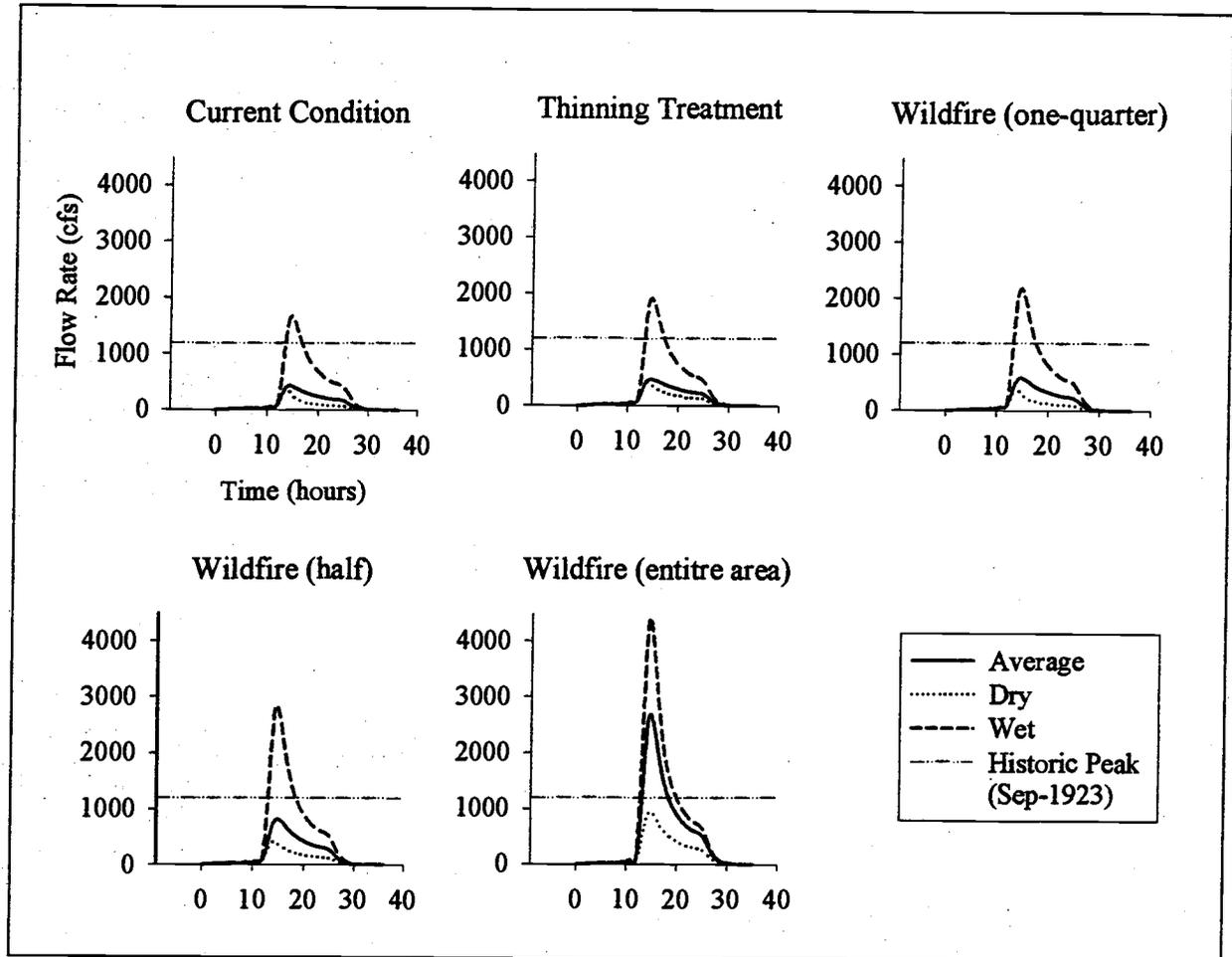
Figure 8. Hydrographs from a 25 yr storm over a wildfire that burned the entire watershed, producing discharge values greater than 2–4 times the historic peak discharge of 1200 cfs under average and wet antecedent soil moisture conditions (AMC). A similar storm over intensely thinned forest and any AMC type produces discharge at least 200 cfs below those over a wildfire that burned one-quarter of the watershed.
