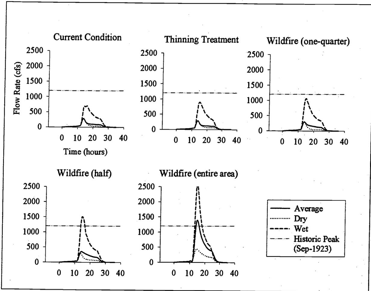
Figure 7. Hydrographs for a 10 yr storm show the peak discharges to be different under varying treatment scenarios and antecedent soil moisture conditions (AMC). The peak discharge following a wildfire that burned the entire watershed is approximately 2500 cfs. Other scenarios under average and dry AMC produce discharges between 300 and 1400 cfs after a 10 yr storm.
