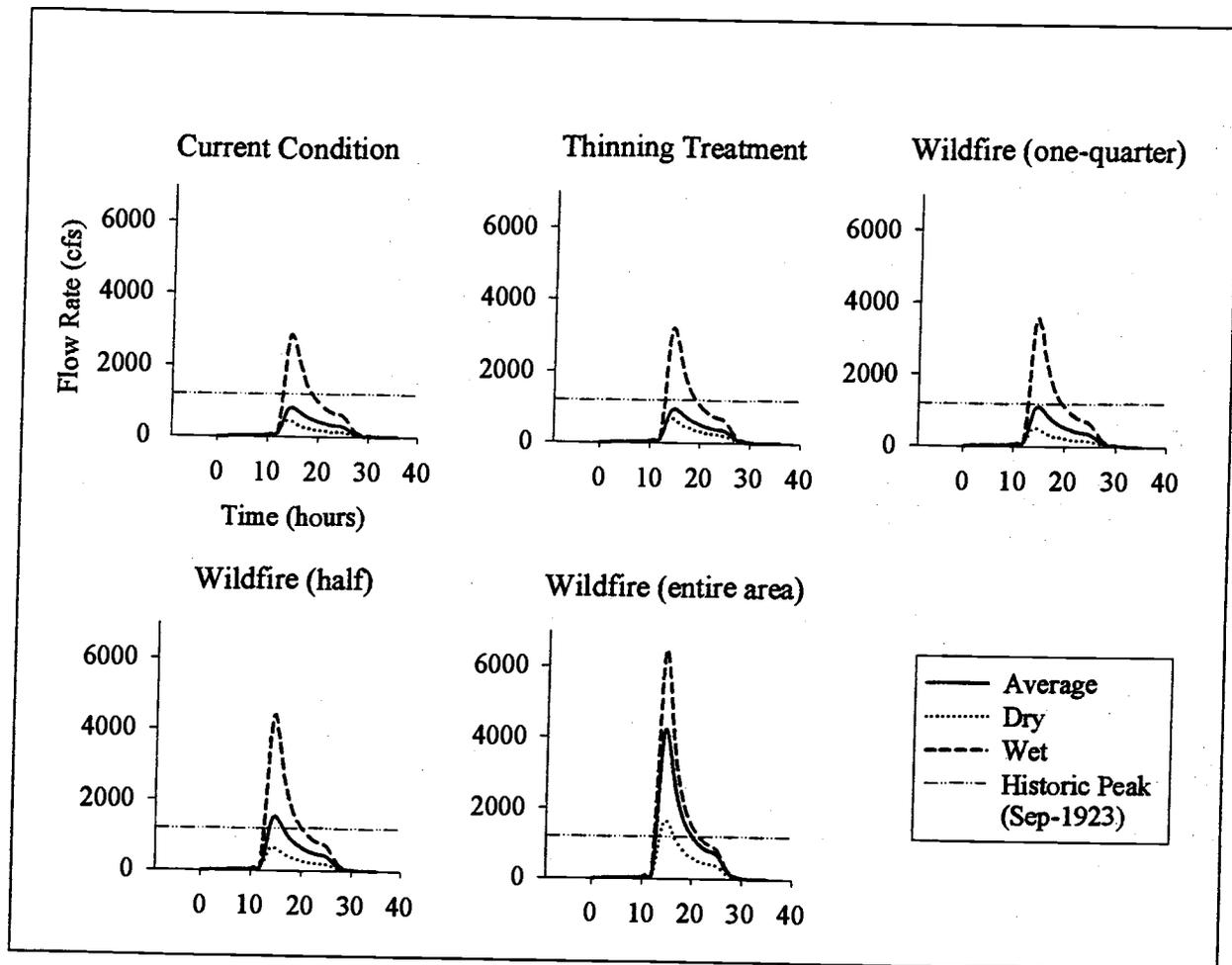
Figure 9. Hydrographs from a 50 yr storm showing a gradual increase with changes in treatment from current condition to wildfire over the entire watershed. Discharge after intense forest thinning is below the smallest wildfire scenario and above the current condition.
