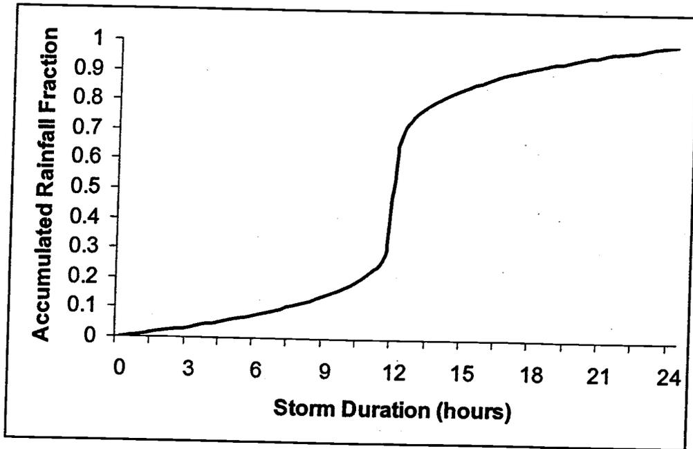
Figure 3. SCS Type II rainfall distribution model for a 24 hour storm (ordinates taken from McCuen 1982).
