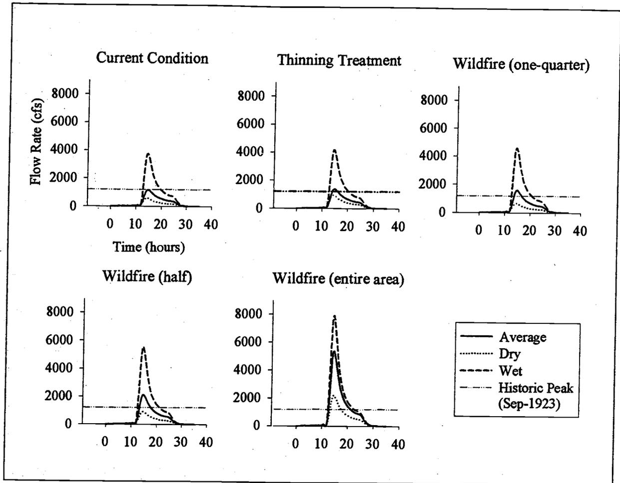
Figure 10. Hydrographs from a 100 yr storm showing peak discharges after a wildfire burned the entire watershed between 2 and 6.5 times greater than the historic peaks in all antecedent soil moisture conditions (AMC). Under average AMC the peak discharge from the current condition is equivalent to the historic mark of 1200 cfs and slightly higher at about 1500 cfs in the intensely thinned forest scenario.
