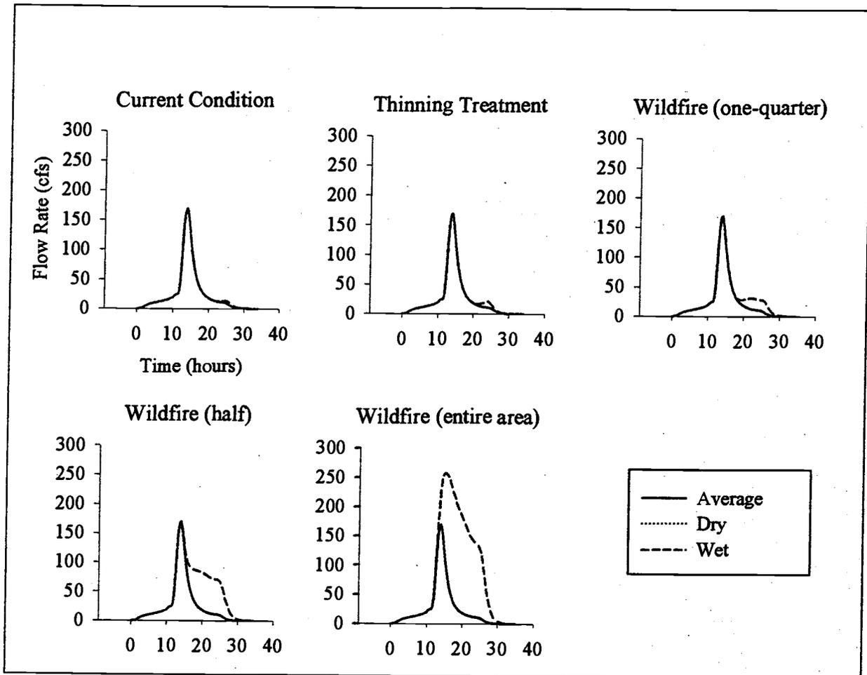
Figure 5. Hydrographs from a 2 yr storm showing peak discharge less than 260 cfs following the worst scenario of entire watershed burn.
