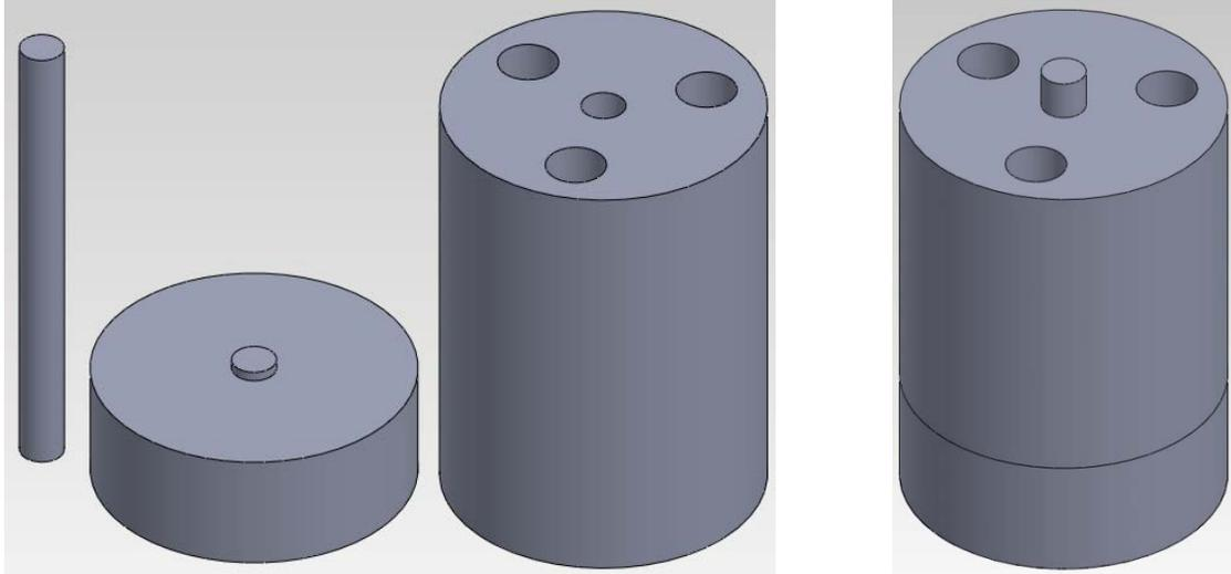
Fig. 1. Solidworks design of the die components (left) and the assembled die (right)
