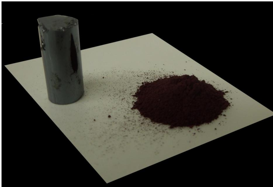
Fig. 5:  $\text{GeSe}_4$  before ball-mill (left) and after ball-mill (right)
