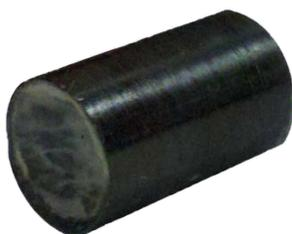
Fig. 6: Sintered GeSe<sub>4</sub> sample from the hot-press system.
