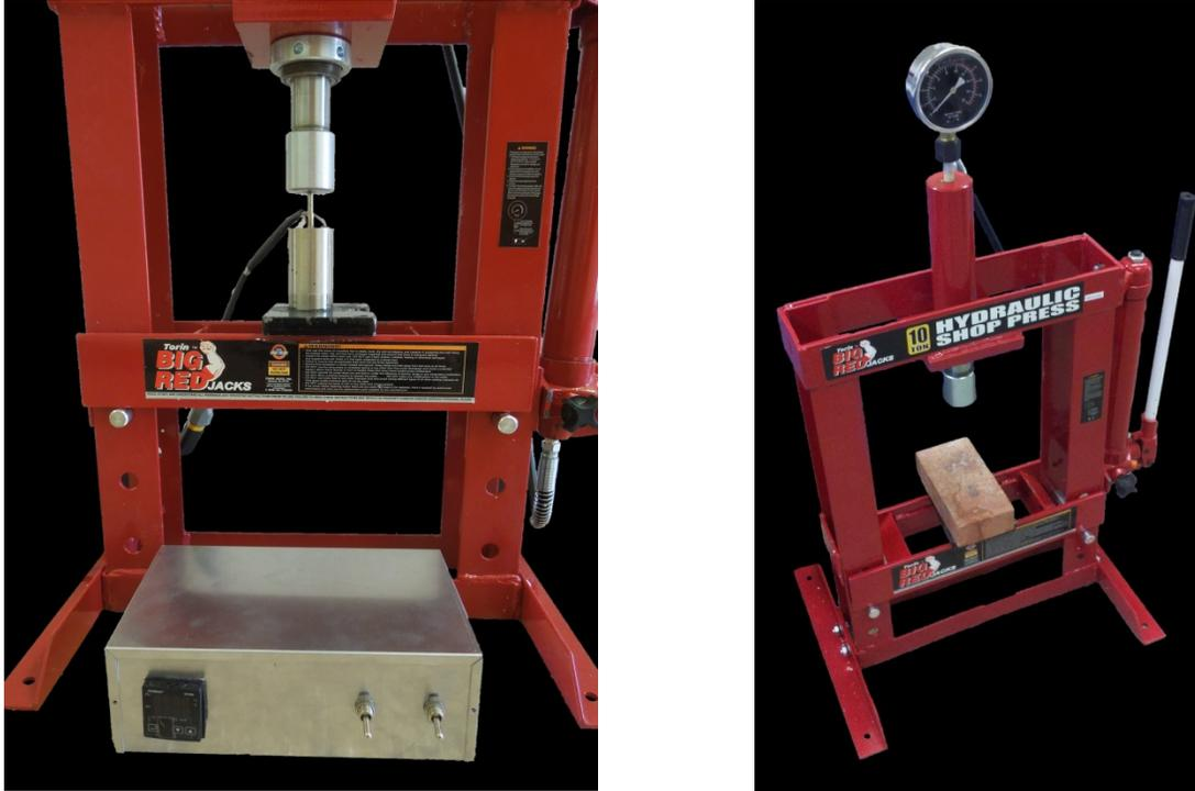
Fig. 2 Full hot-press setup (left) and the press standing alone (right)
