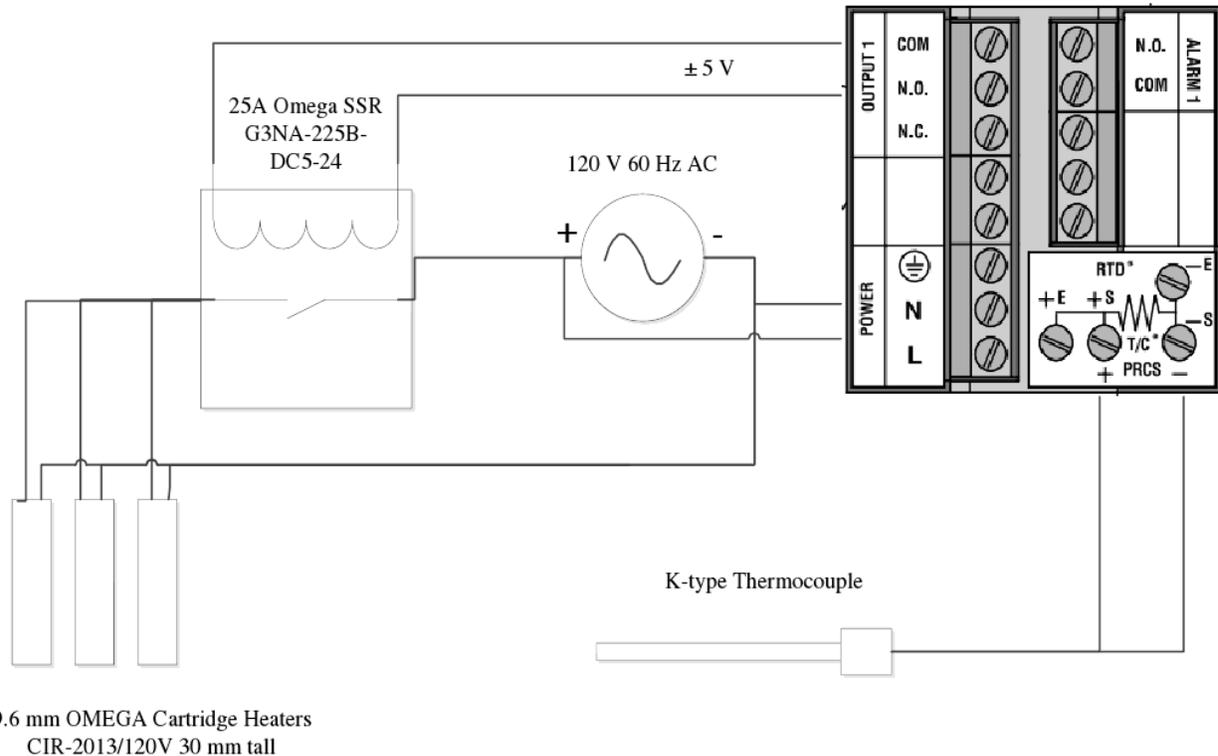
Fig. 4: Electrical Diagram including the PID controller in the upper right, the solid-state relay located at the upper left, and the OMEGA heating cartridges in the bottom left.
