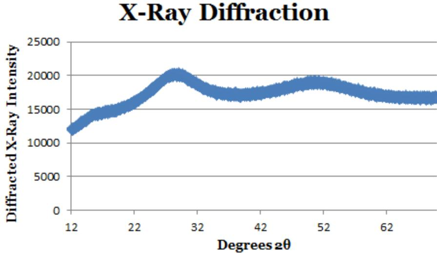
Fig. 7: XRD results of the GeSe<sub>4</sub> sintered sample showing no crystalline peaks.
