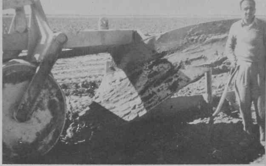
▲ This giant moldboard plow (above) is used to plow soils up to depths of 30 inches.
