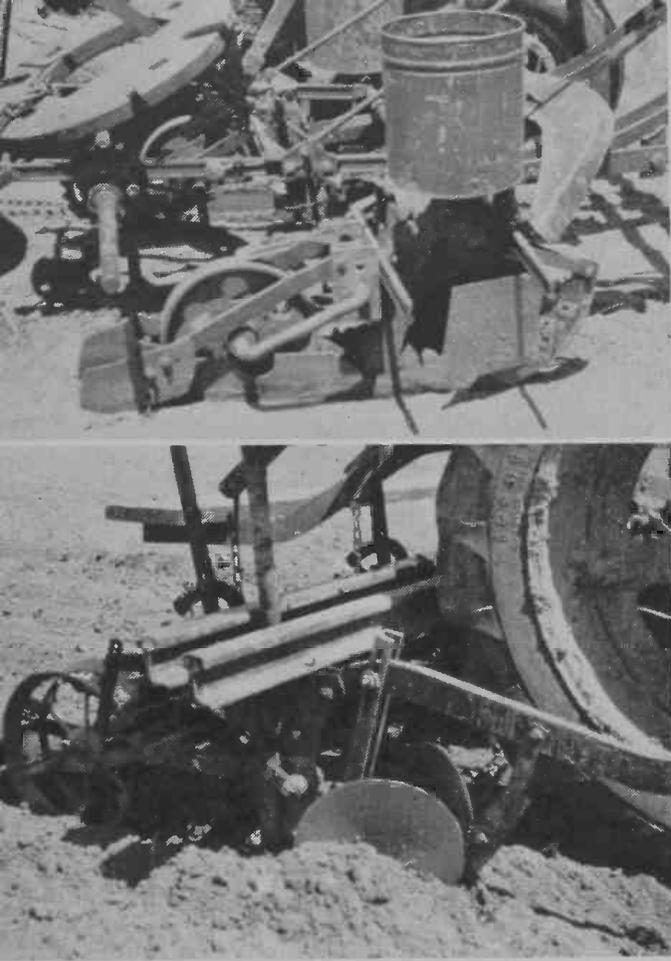
Above: Milled packer wheel to force seed into moist ground before coverage. Useful on clay ground that dries out badly. Note weights to force planter into these heavy soils.
