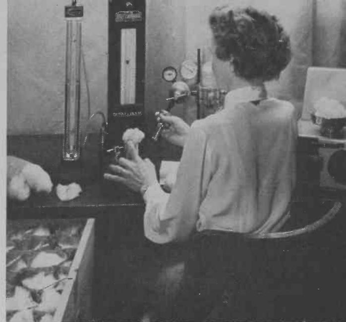
Cover Picture — Using the Microneaire to test individual plant selections for fineness of fiber. This instrument is used extensively by spinners in making up their blends.
