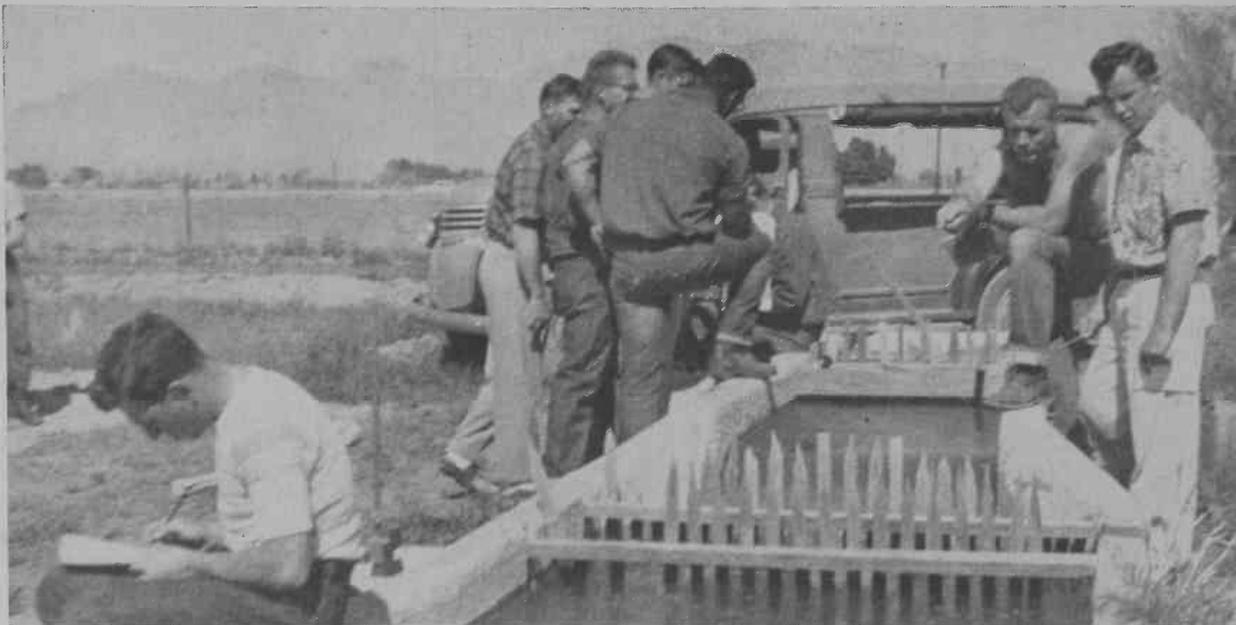
Field exercise in the measurement of irrigation water through a Cippolletti weir, a suppressed rectangular weir, a submerged orifice, and a Parshall flume.
