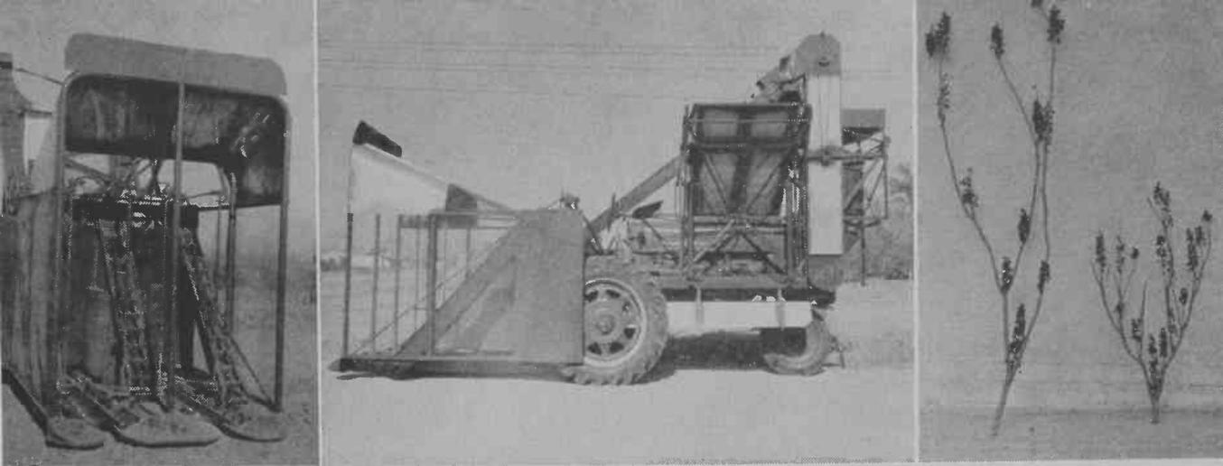
LEFT TO RIGHT are, 1—Front view of tractor-mounted castor bean harvester manufactured in Arizona; 2—Side view of same machine; and 3—Normal size plant of U. S. Hybrid 415 and, at its right, ← the dwarf castor bean plant which is only four feet high. The present breeding program seeks to develop a high-yielding dwarf castor bean which can be easily machine-harvested.
