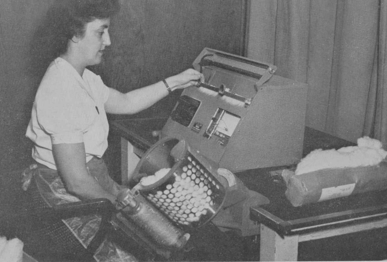
IN THE UA cotton laboratory, Mrs. Doris Waterworth is preparing to run a cotton sample on the fibrograph to measure length of the sample. The instrument at her right, a cylinder containing cotton, is the fibro-sampler.
