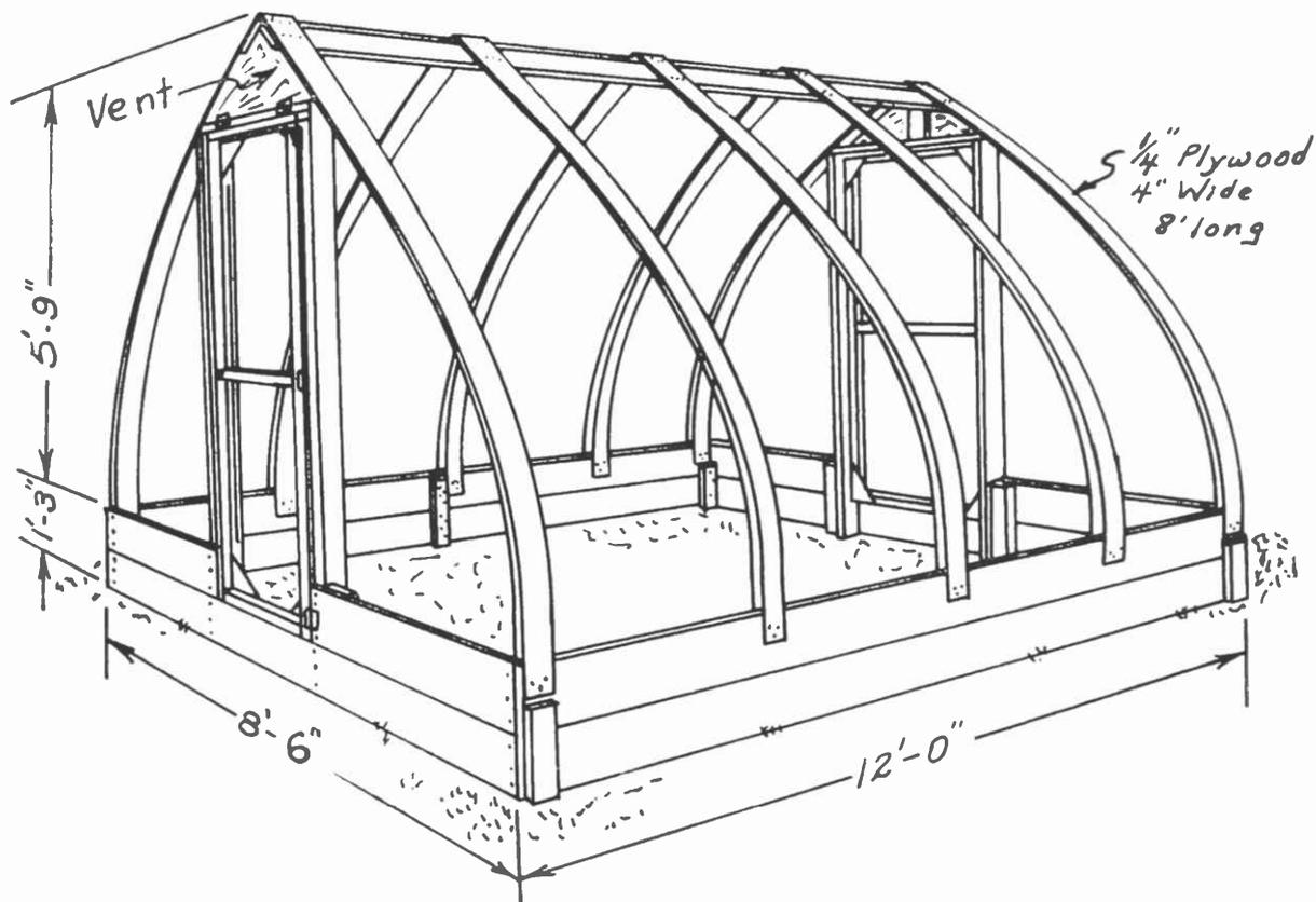
**PERSPECTIVE OF GREENHOUSE, Plan 5946, shows how baseboards are installed, also plywood arches and ridge-board. For actual working drawings, apply at your local County Agent's office.**
