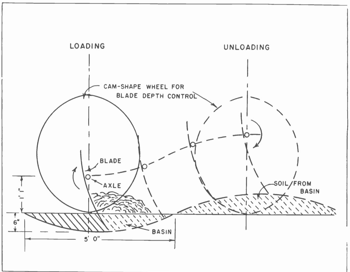
GRAPH ABOVE SHOWS blade and depth-control cam wheel for forming basins, showing basins and soil deposited between basins.
