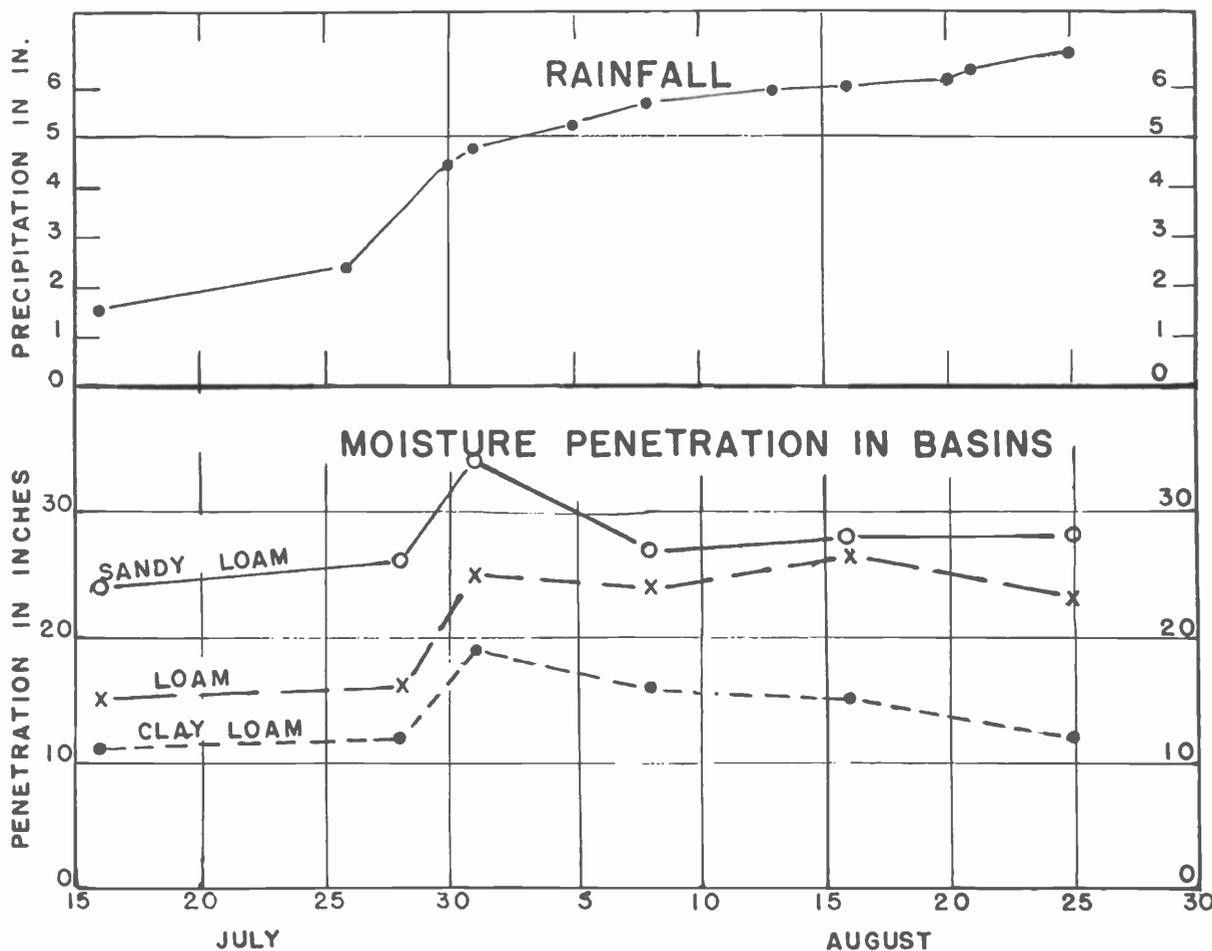
**GRAPH ABOVE SHOWS 1963 summer rainfall and cumulative moisture penetration in basins on the Santa Rita Experimental Range. Note differences caused by different soil types.**
