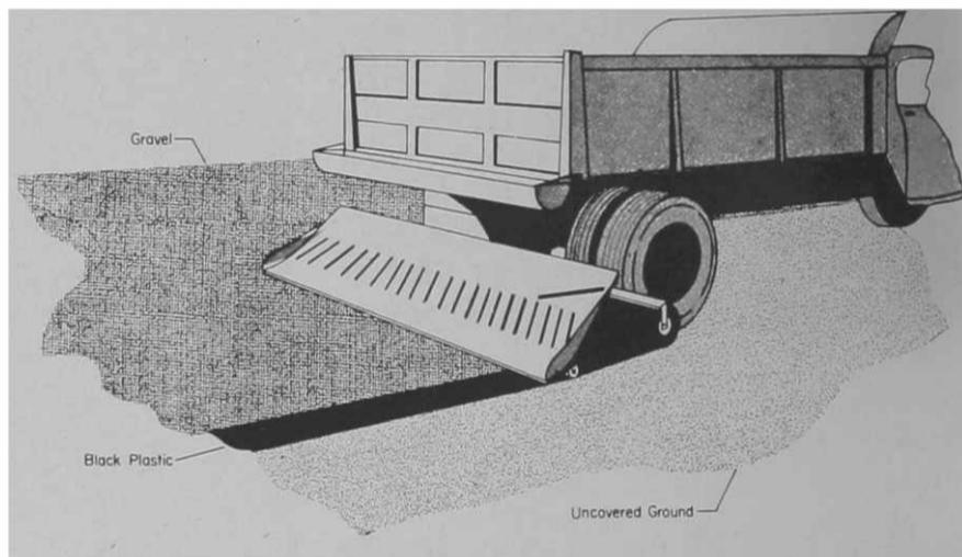
**ARTIST'S DRAWING** shows how the plastic-laying gravel spreader operates.
