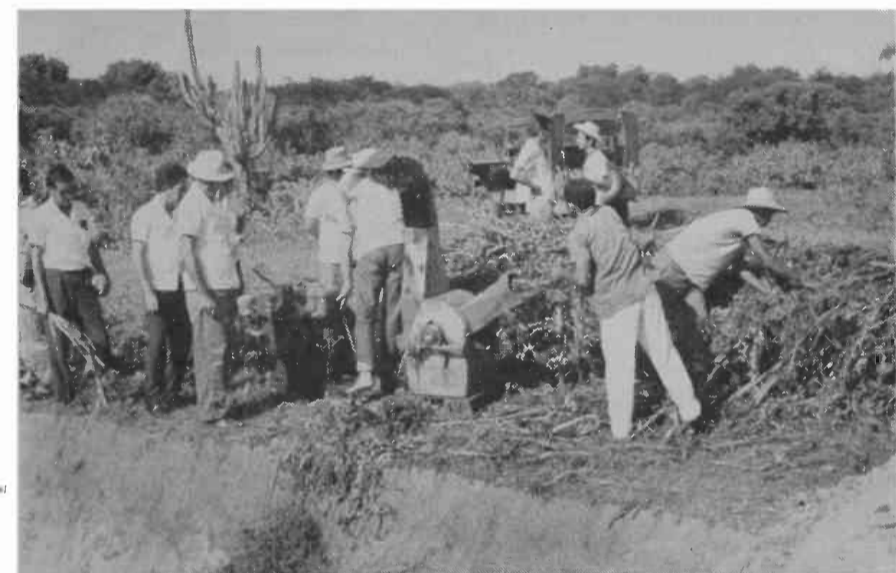
SMALL GASOLINE-POWERED stationery chopper is used to slowly fill a trench silo. Forage is cut by hand and hauled to the chopper on burros or on small carts. While slow and awkward by North American standards, this represents a great step forward in a drought-susceptible area where no livestock feeds of any kind were preserved up to the present time.
