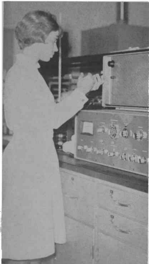
GAS CHROMATOGRAPHY is used as a tool by the Division of Food and Nutrition. Here Student Martina Cooper injects fatty acid methyl extract into the chromatograph.
