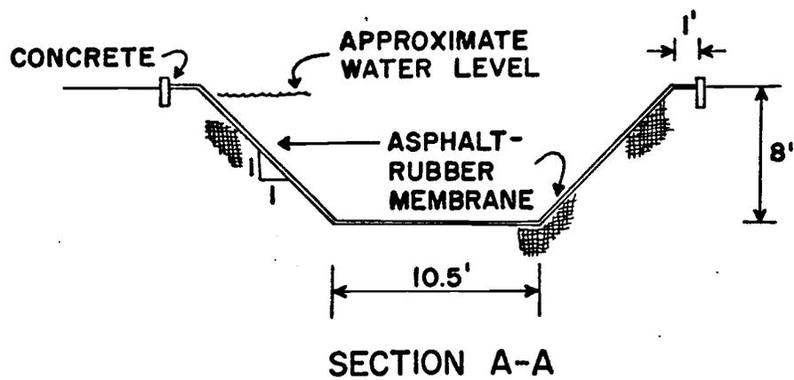
Figure 15. Reservoir Used for Asphalt-Rubber Membrane Lining
