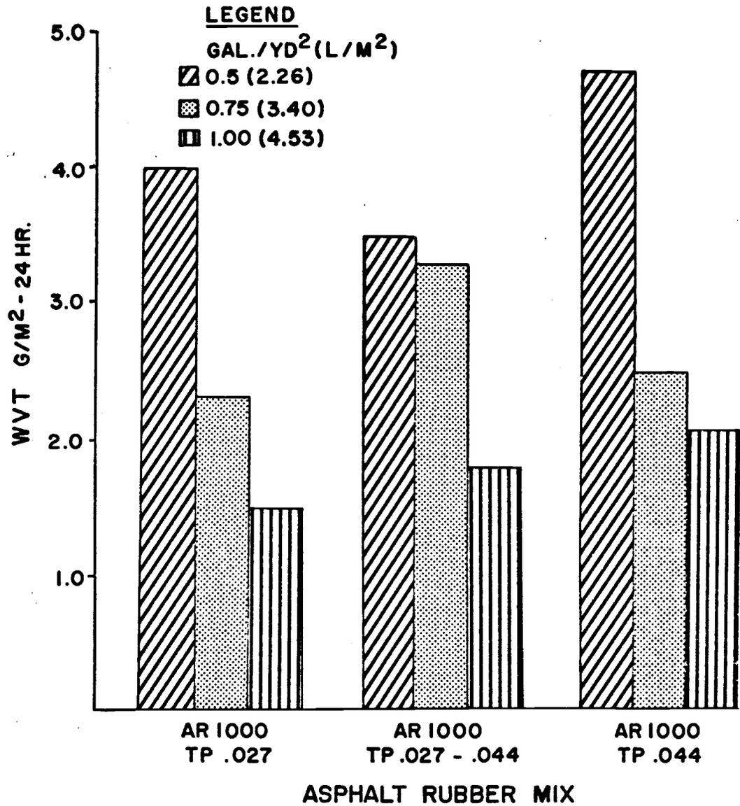
Figure 12. Relative WVT Rates for Various Asphalt-Rubber Mixes
