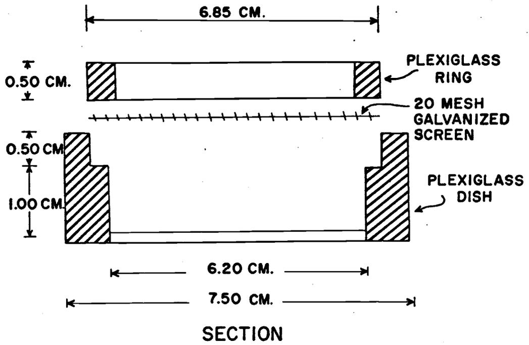
Figure 2. Water Vapor Transmission Test Dish
