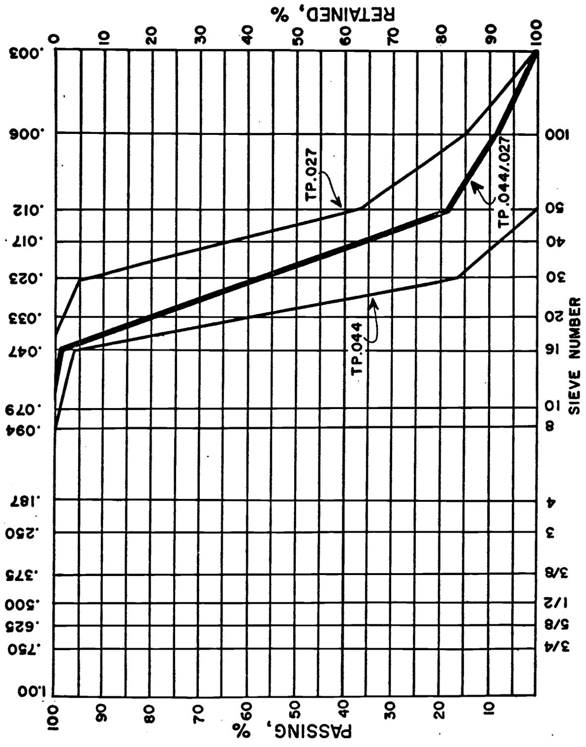
Figure I - 1. Particle Size Distribution of Crumb Rubber Used in the Asphalt-Rubber Testing.
