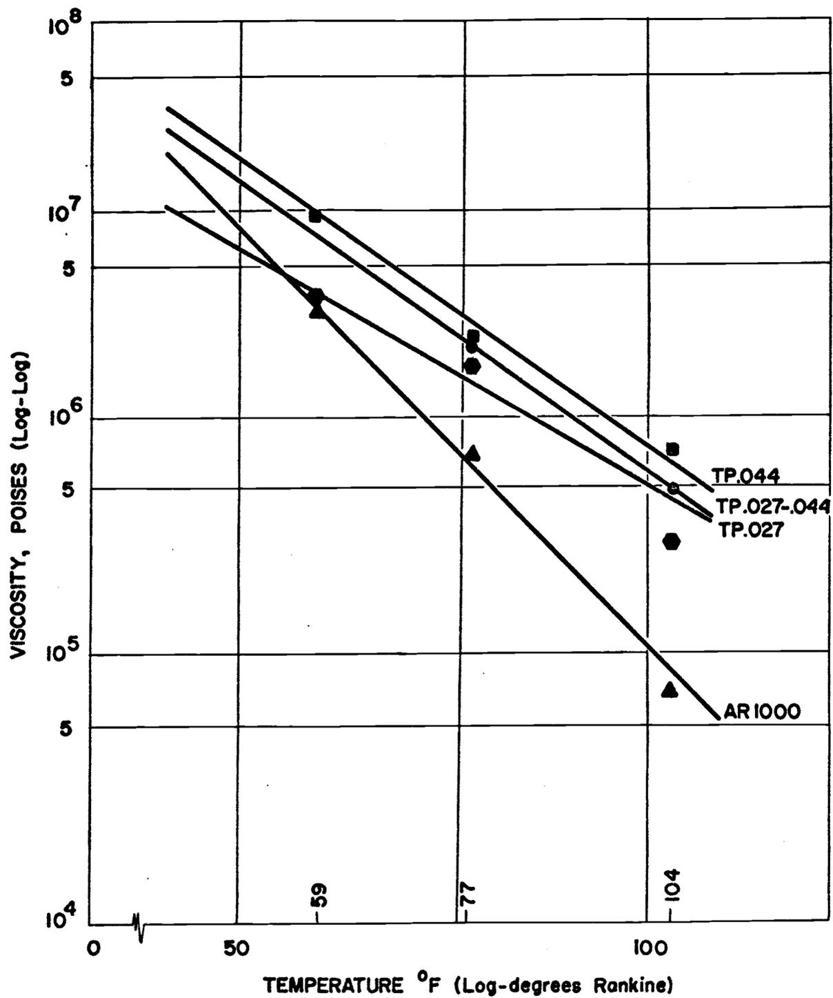
Figure 10. Effect of Temperature on the Viscosity of Asphalt and Asphalt-Rubber Mixtures
