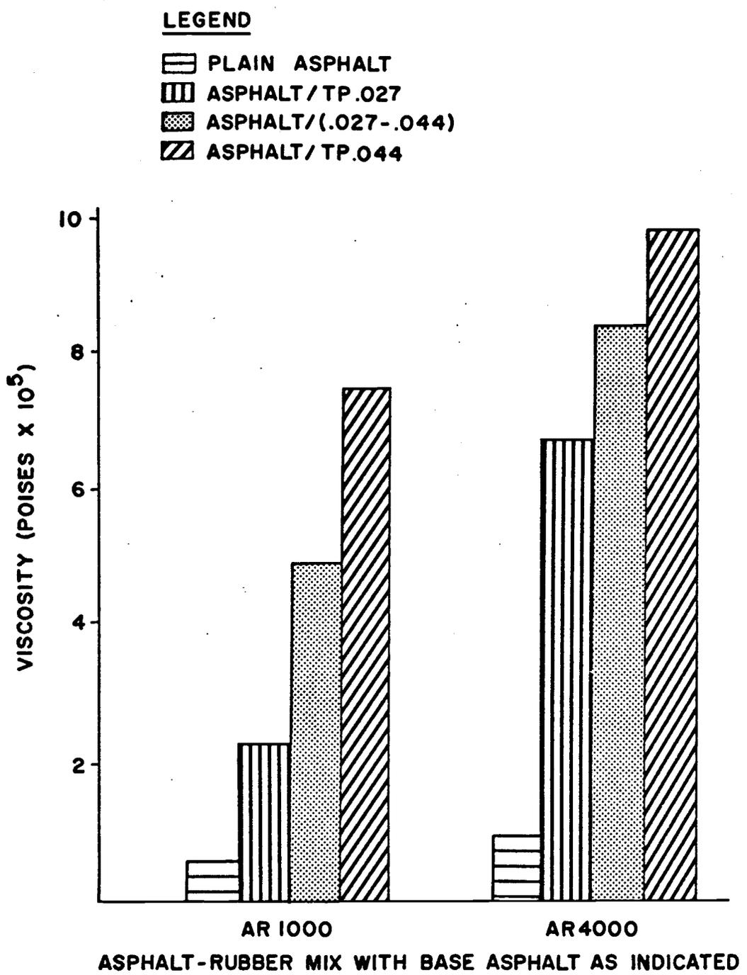
Figure 9. Relative Viscosities of Asphalt-Rubber Mixes at 104°F (60°C)
