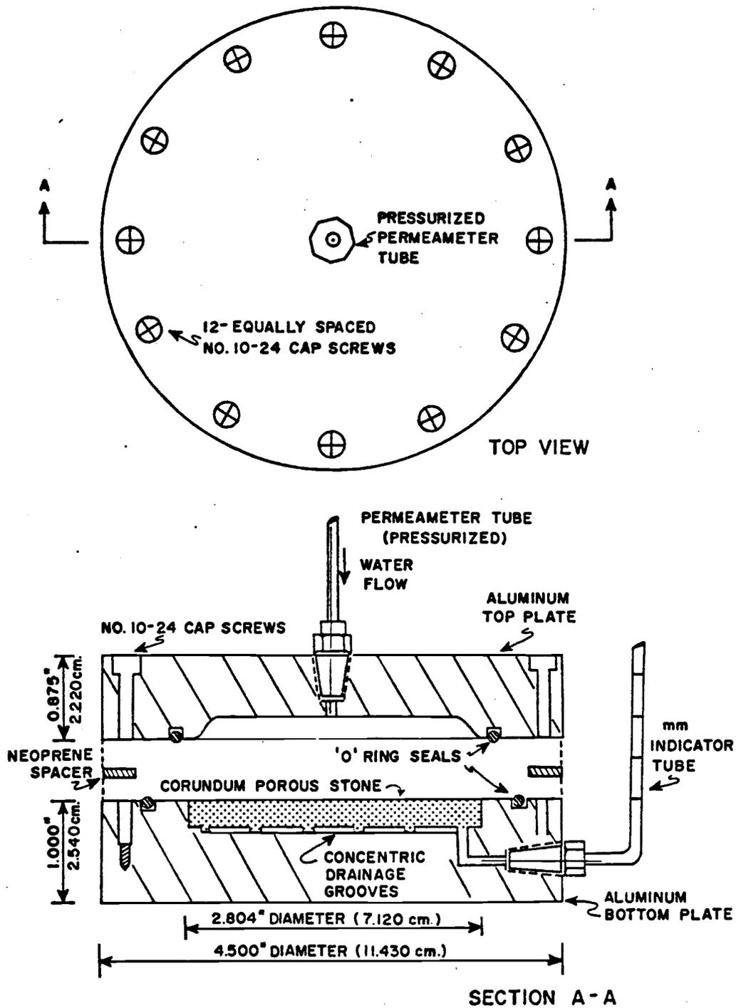
Figure 5. Static Head Permeameter
