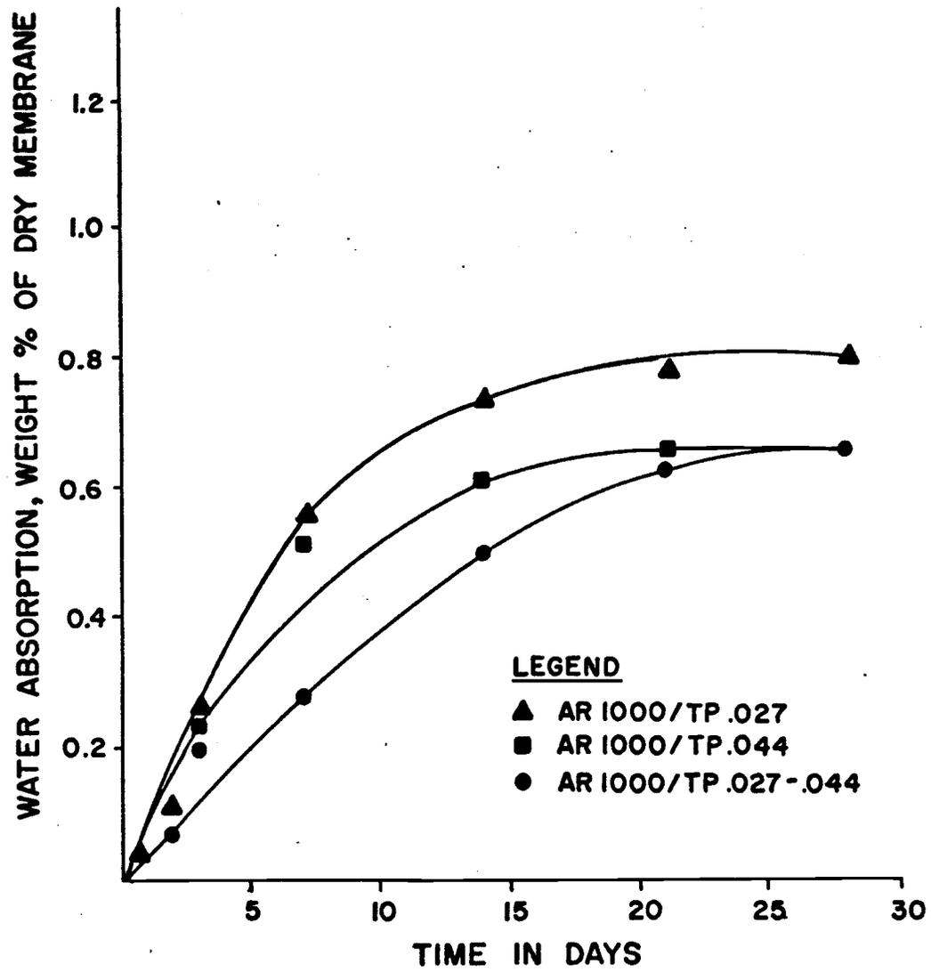
Figure 13. Relative Water Absorption Rates for Various Asphalt-Rubber Mixes
