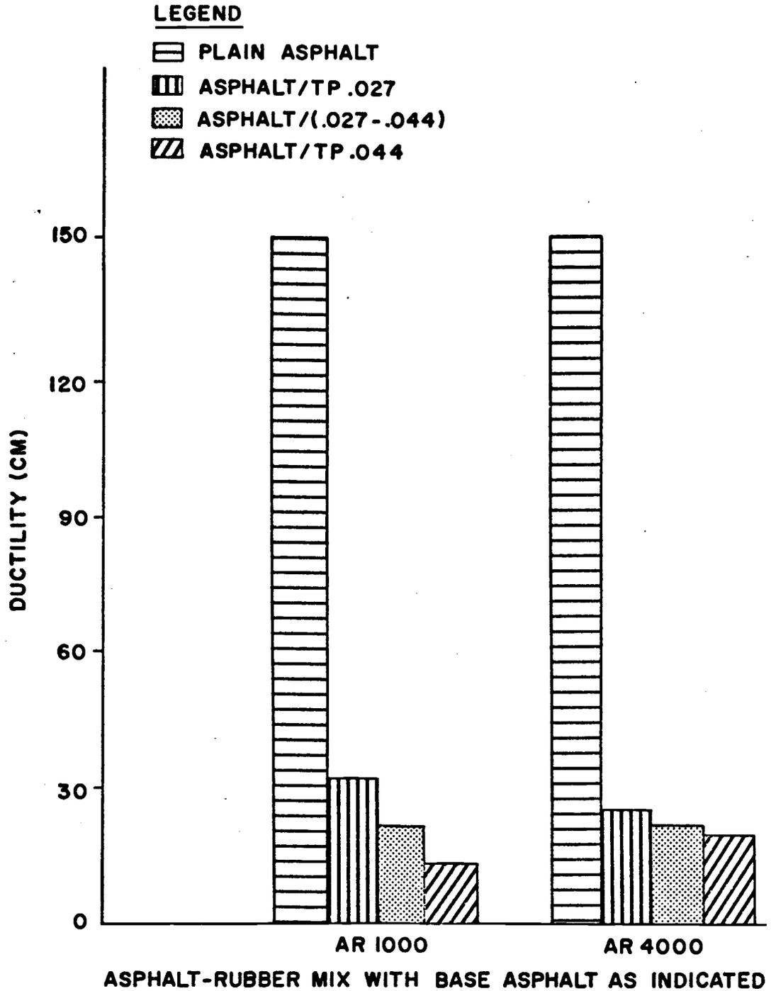
Figure 11. Ductility Values for Asphalt and Asphalt-Rubber Tested at 77°F (25°C).
