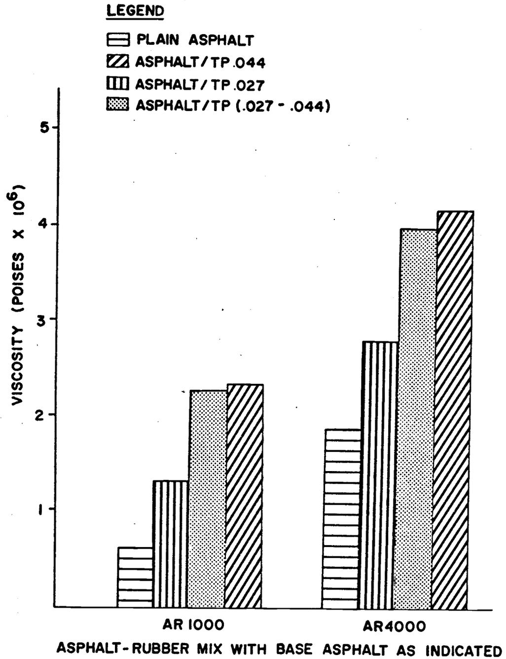
Figure 8. Relative Viscosities of Asphalt-Rubber Mixes at 77°F (25°C)
