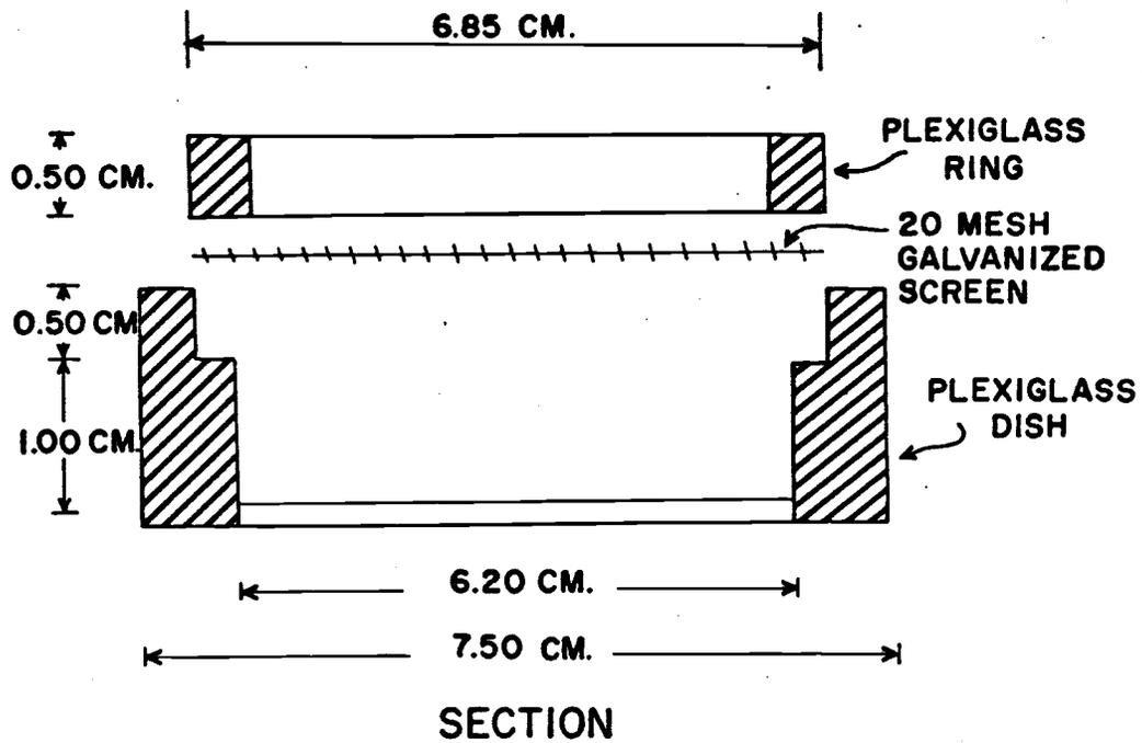
Figure 2. Water Vapor Transmission Test Dish
