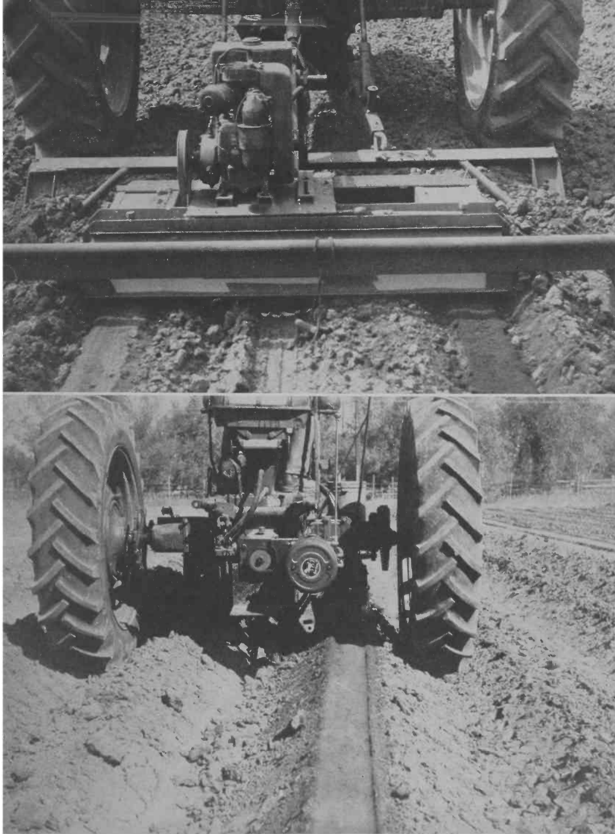
FIGURE 3. (Top) Grinder-type mulcher operated by gasoline engine and used for preparing surface for asphalt emulsion for dry planting. (Bottom) Strip of soil surface prepared by grinder-type mulcher for emulsion application.
