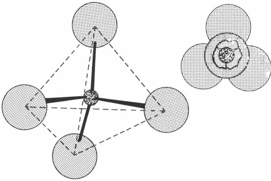
1. Model of a single silicon-oxygen tetrahedron. The perspective, expanded view, left, and cutaway view, right. Three of the oxygen atoms lie in a single plane while the fourth extends above this plane.
