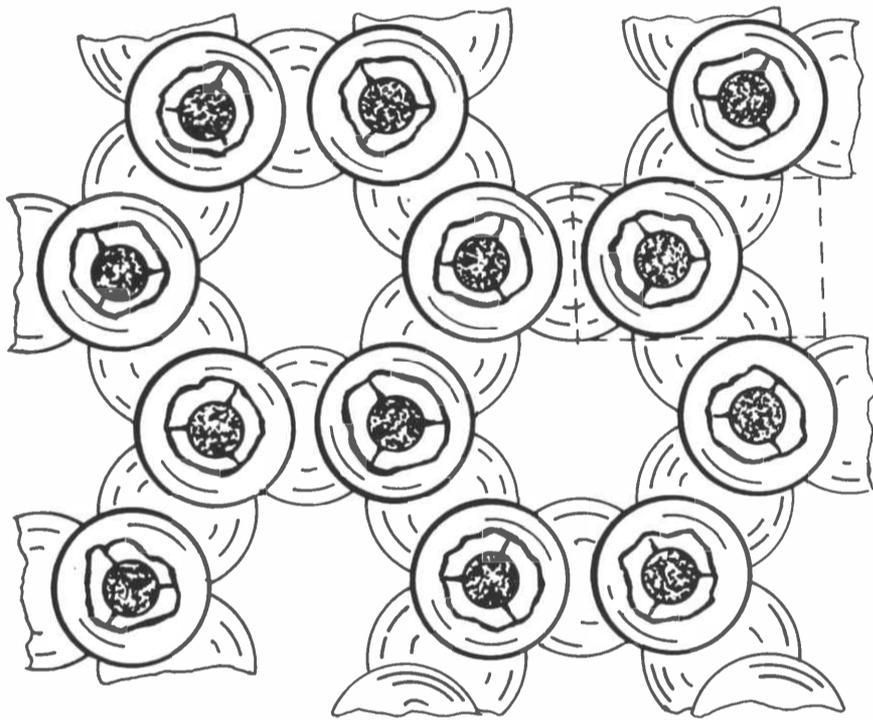
2. Twelve silicon-oxygen tetrahedrons joined together to illustrate the sheet-like structure of mica. This model illustrates the way in which the silicon atoms (darkened spheres) share the oxygen atoms (larger spheres) lying in the horizontal plane.
