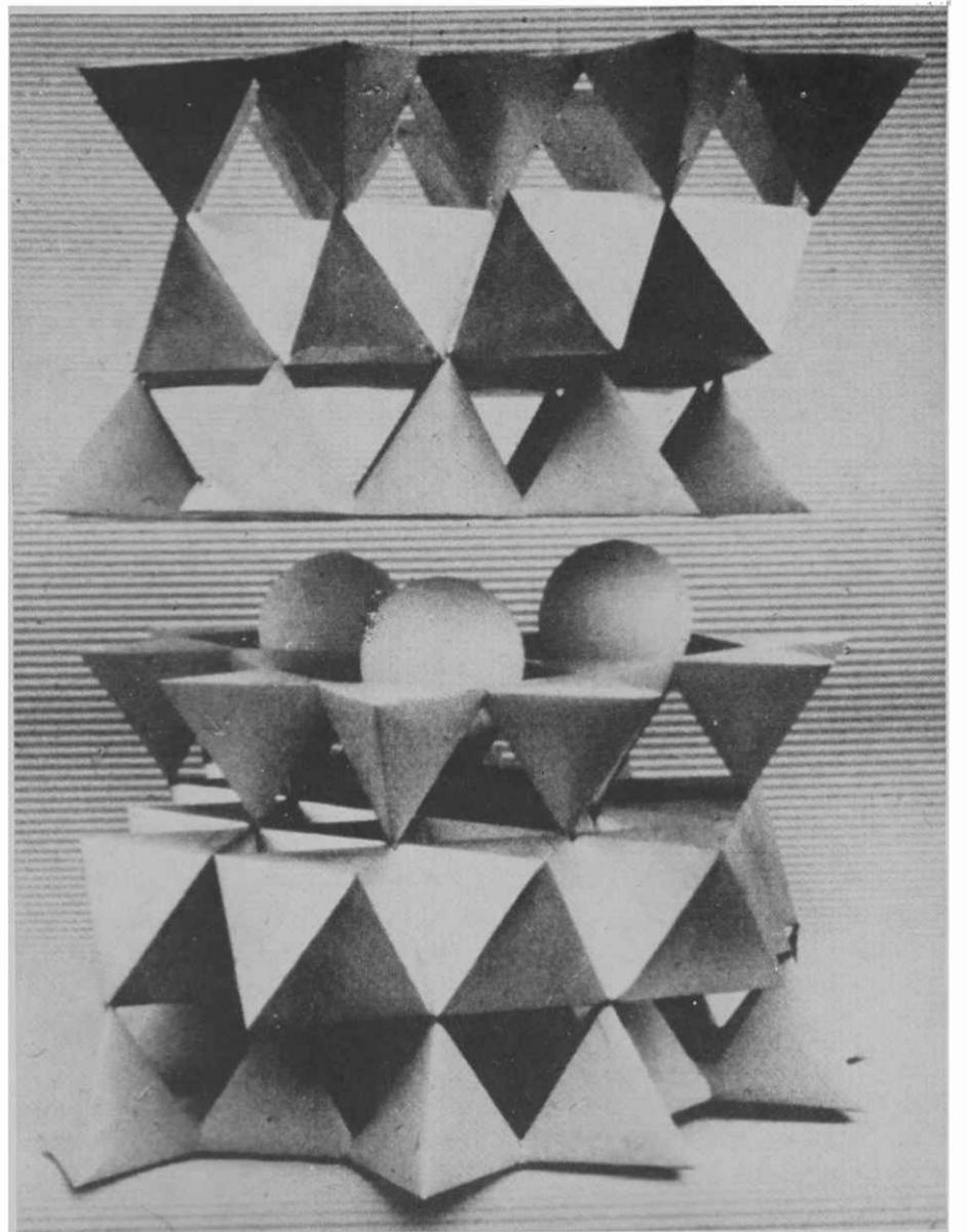
3. Structural model of mica showing the tetrahedron-octahedron arrangement. The white balls show the position of potassium ions in openings in the surface of the silicate.
