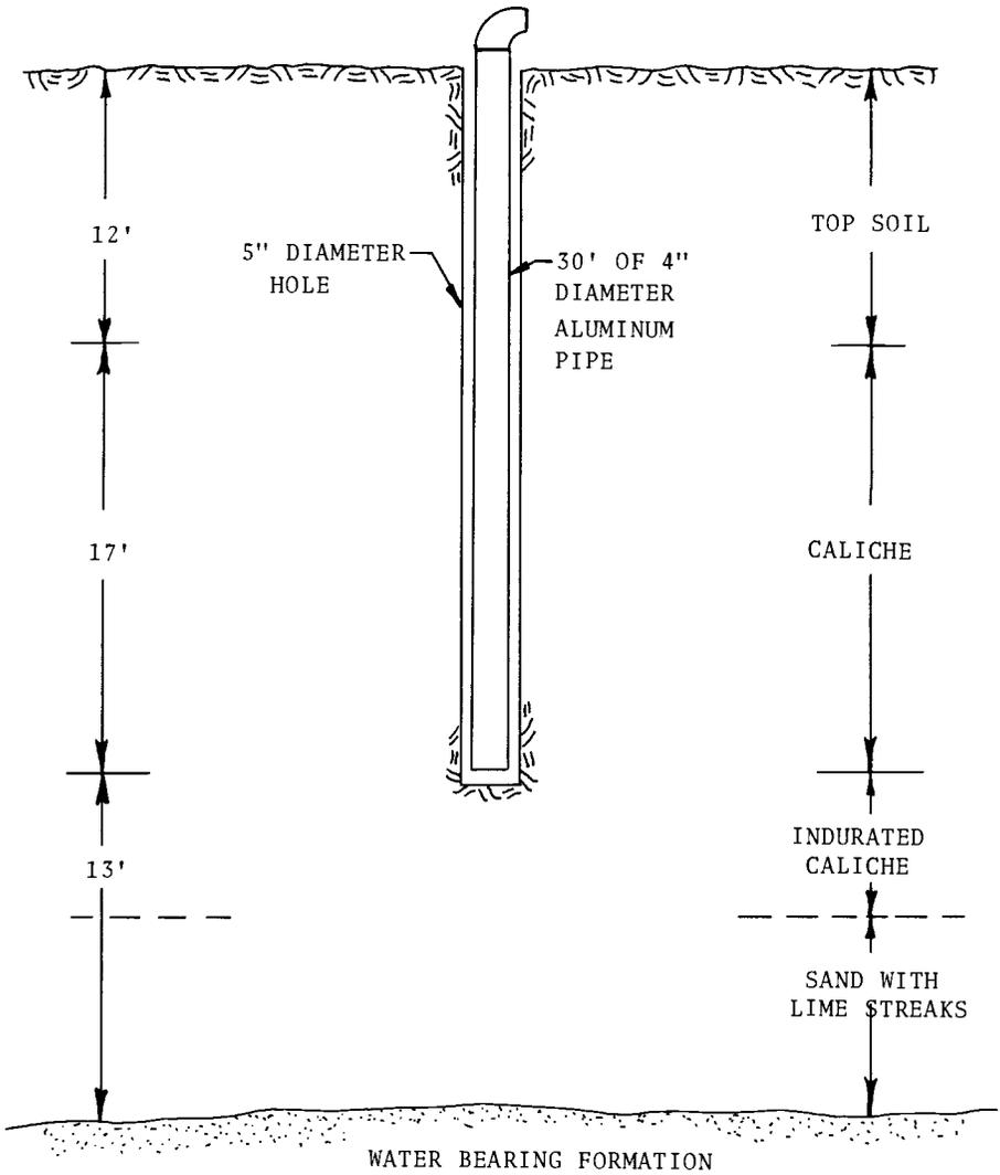
Figure 4. Schematic of the initial hole recharge facility.
