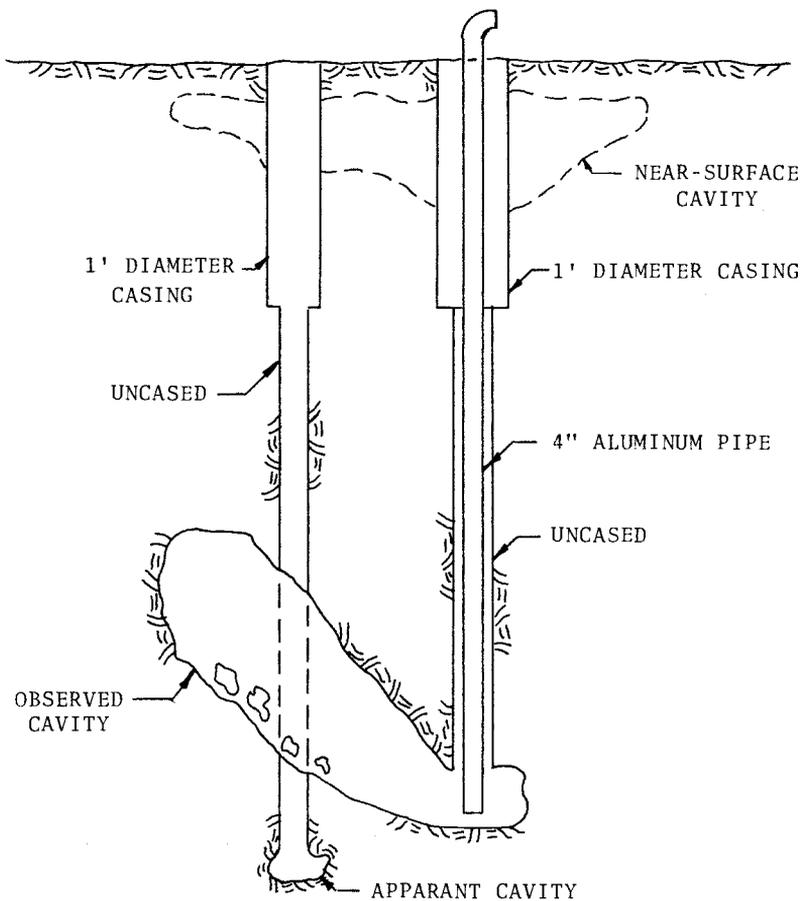
Figure 5. Schematic of cavity at base of hole, March, 1970.
