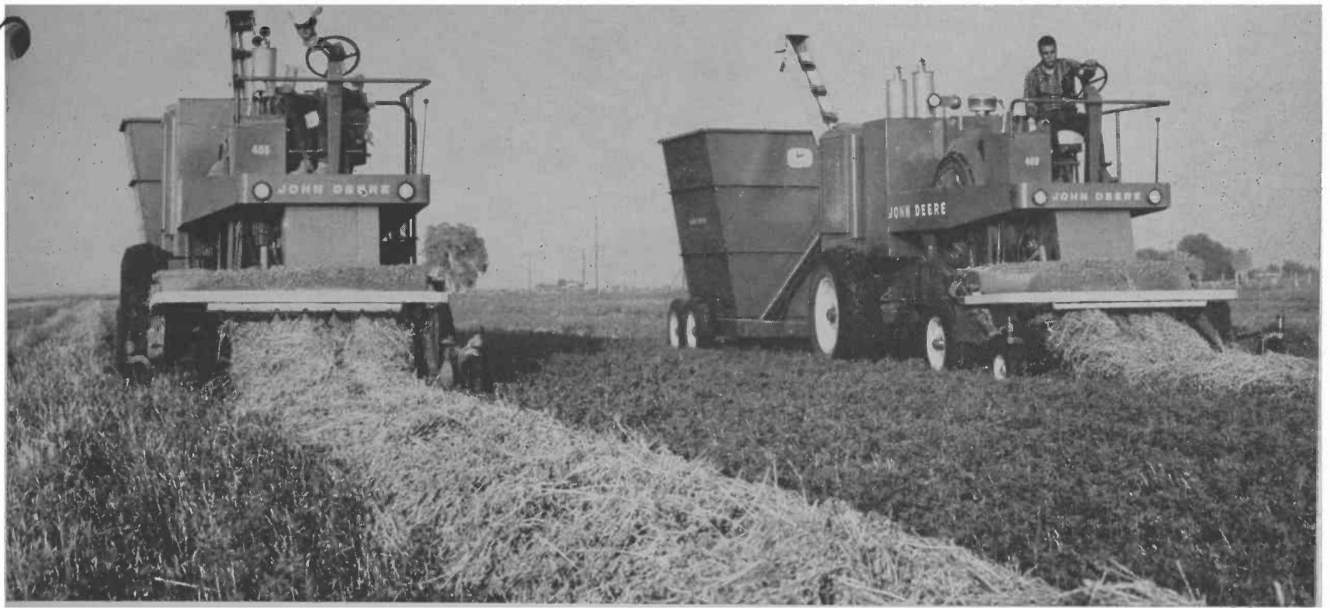
Figure 2. In this picture as well as on the cover is shown hay cubing machines picking up cured hay after being mowed and windrowed. Note the sprays of water being applied to the hay as it is being picked up. This is done to bring the hay to proper moisture content for good compaction in the cubing process.
