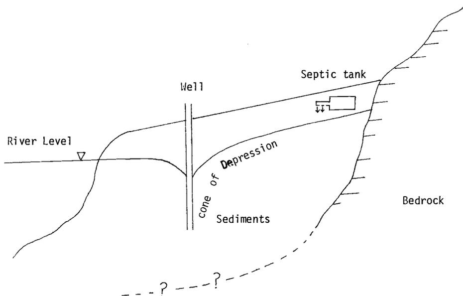
FIGURE 4. Relationship Between River, Wells, and Septic Tanks
