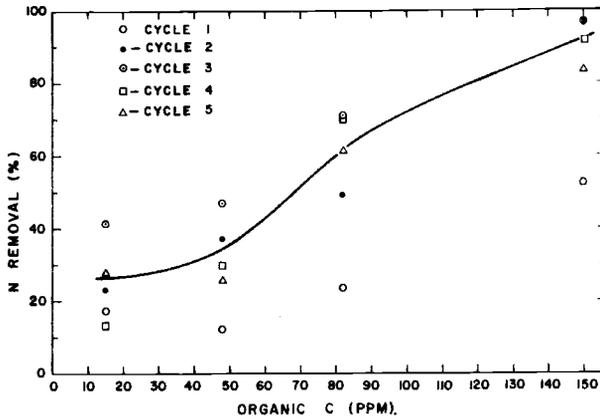
Fig. 1. The effect of the organic carbon content of secondary sewage effluent on nitrogen removal from the sewage by soil columns flooded on cycles of 9-day flooding and 5-day drying. Dextrose was added to the sewage water to provide levels of organic C.
