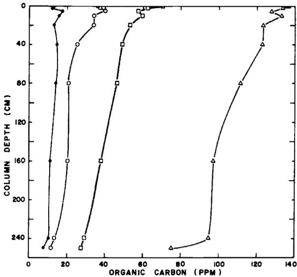
Fig. 2. Organic carbon concentrations of samples from various depths along soil columns flooded with secondary sewage effluent supplemented with different levels of organic carbon as dextrose. (Average organic C concentrations entering the columns were 15(●), 40(○), 80(□), and 150(△) ppm.
