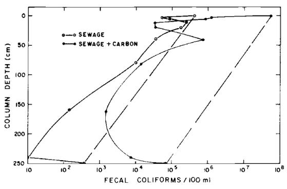
Fig. 4. Fecal coliform counts of samples from various depths along soil columns flooded with secondary sewage effluent supplemented with organic carbon as dextrose.
