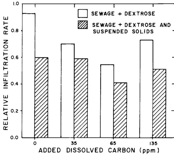
Fig. 3. Relative infiltration rates of soil columns flooded with secondary sewage effluent. Average rates during a base period when all columns were flooded with sewage only were taken as 1.0. Total carbon concentrations were 15, 50, 80, and 150 ppm, and the base period rates for the columns used for the different treatments were 59, 51, 49, and 59 cm/day, respectively.
