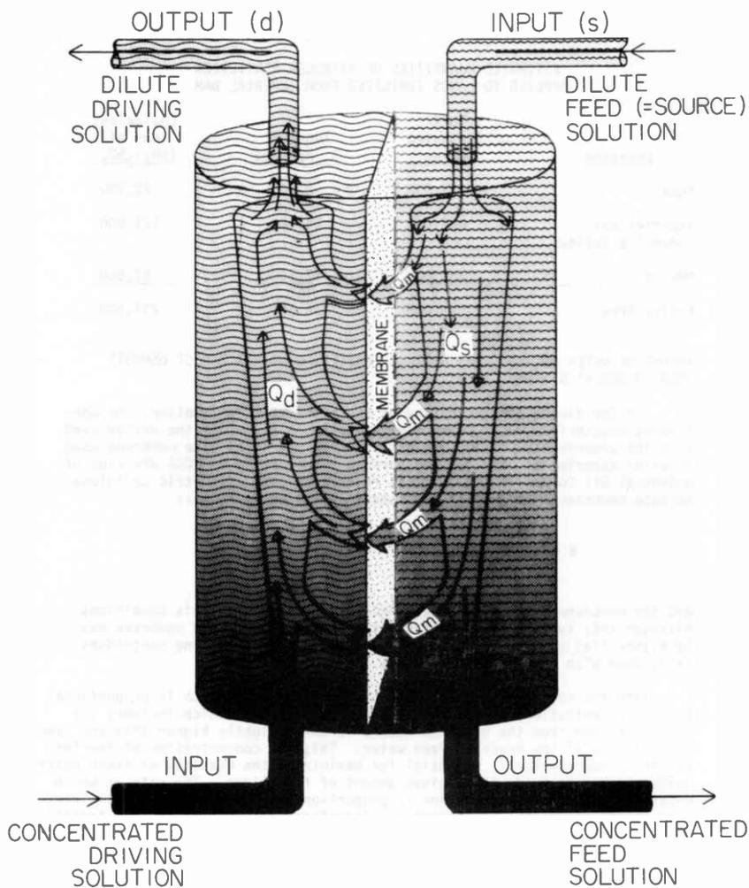
Fig. 1 Schematic view of continuous flow countercurrent extractor.  $Q_s$ ,  $Q_d$  and  $Q_m$  are the feed (=source) and driving solution currents, and the membrane current. The density of shading symbolizes solute concentration, the width of the streams, current magnitudes.
