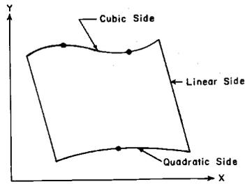
Figure 1. Deformed Mixed Isoparametric Quadrilateral Element. (After Pinder, *ibid.*)
