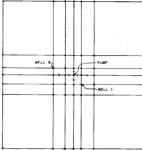
Figure 2. Finite Element Grid for Analysis of two week discharge test.
