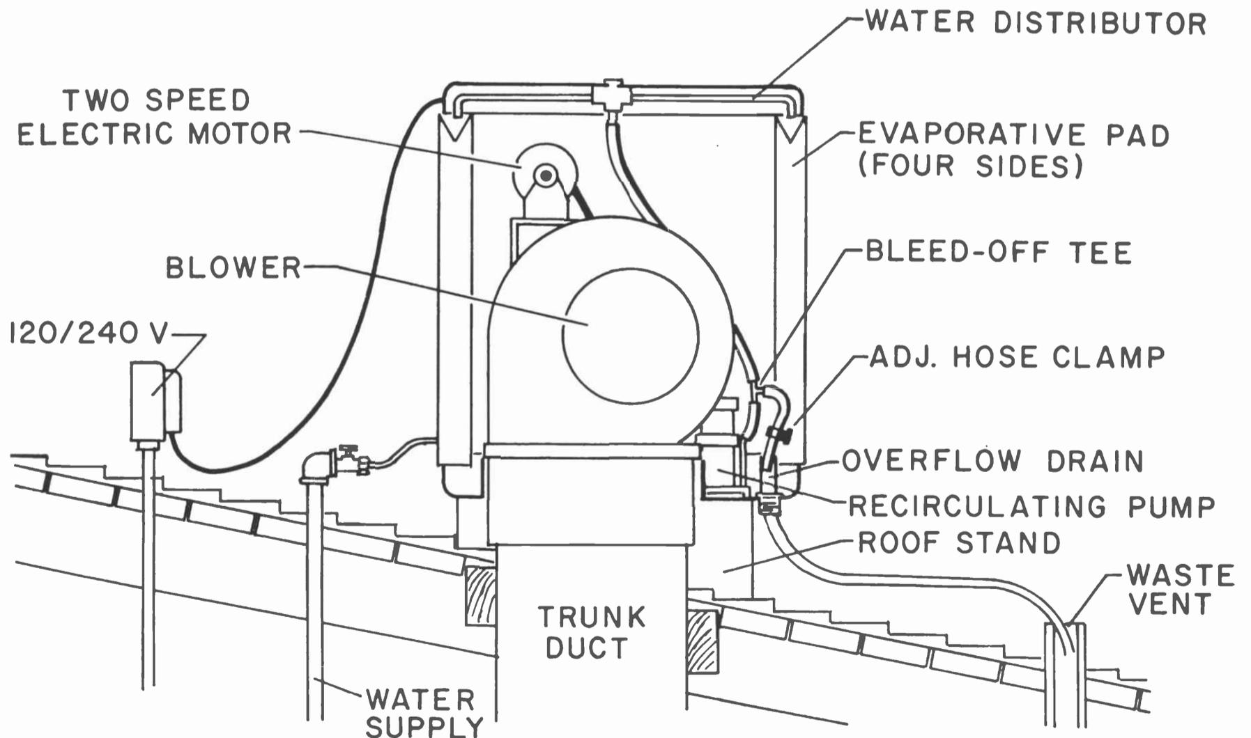
Figure 1. Typical Wet Pad Evaporative Air Conditioner.
