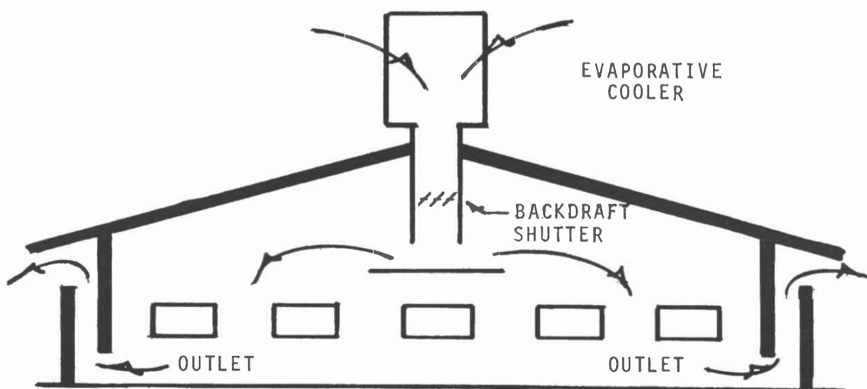
Figure 1. Package Cooled - Cavity Wall System
