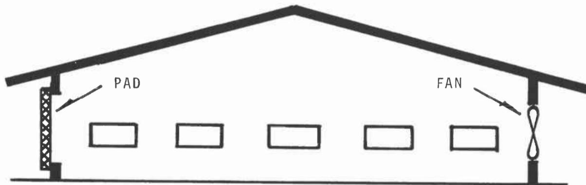
Figure 3 Schematic Pad and Fan System
