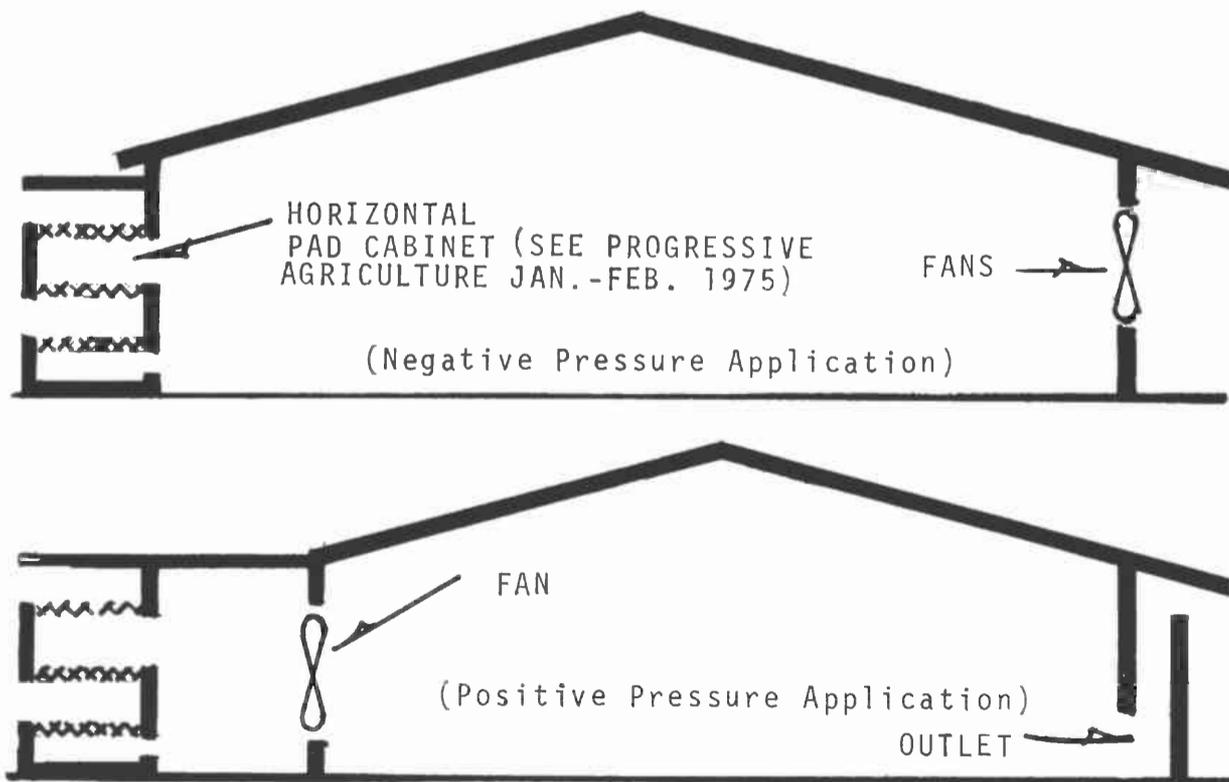
Figure 4. Schematic Horizontal Pad Cabinet Applications.
