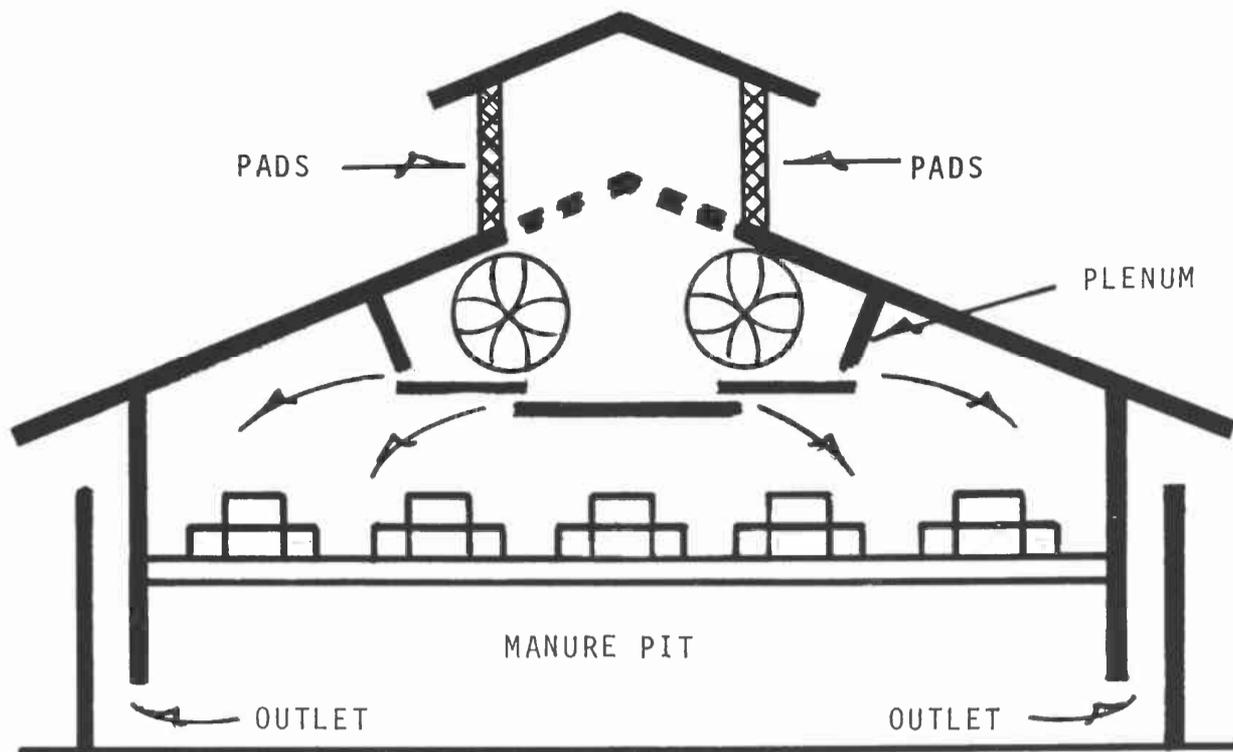
Figure 2 Schematic Tower and Plenum System with Deep Pit
