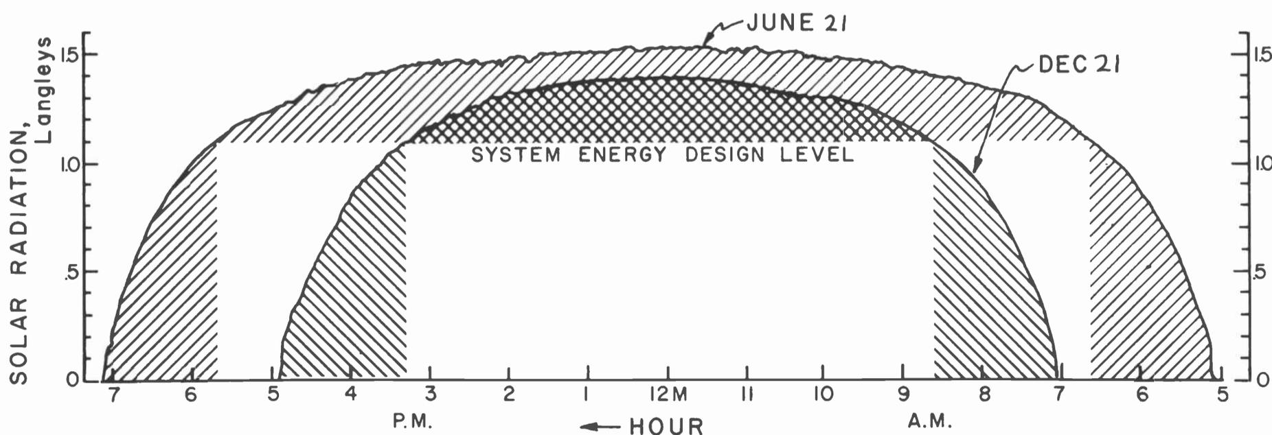
THE FIGURE above shows solar data recorded for the greatest and least amounts of solar radiation that may be expected in Southern Arizona. The dates represent the summer and winter solstices, and the white areas within the shaded areas represent the time during which a solar energy system could function efficiently.
