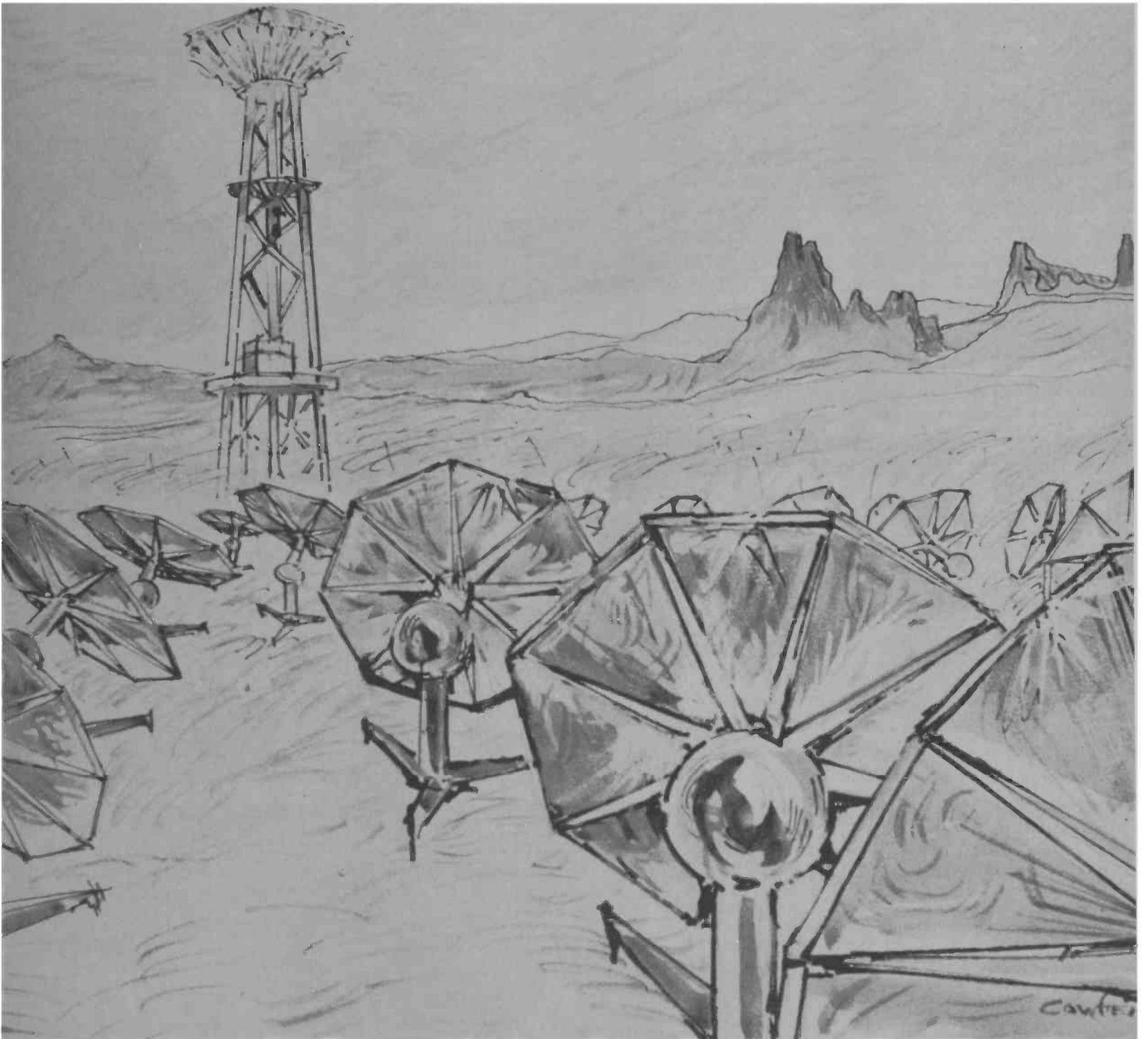
*THIS CONCEPTION of a solar tower collector shows the reflectors surrounding the tower concentrating the sun's rays on the top of the tower. Such a tower is to be built for experimentation at the Sandia Laboratories in New Mexico.*
