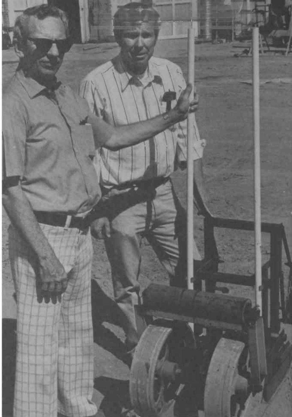
*THE MEN and their machine (Sharples on left, Gentry on right). The seed tablets are contained in the dual plastic pipes, and placed alternately in two rows. The tablets are by Sharples, the machine by Gentry.*
