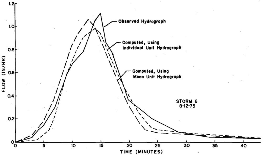
Fig. 6 -- Observed and computed runoff hydrographs for storm of Aug. 12, 1975 (No. 6).
