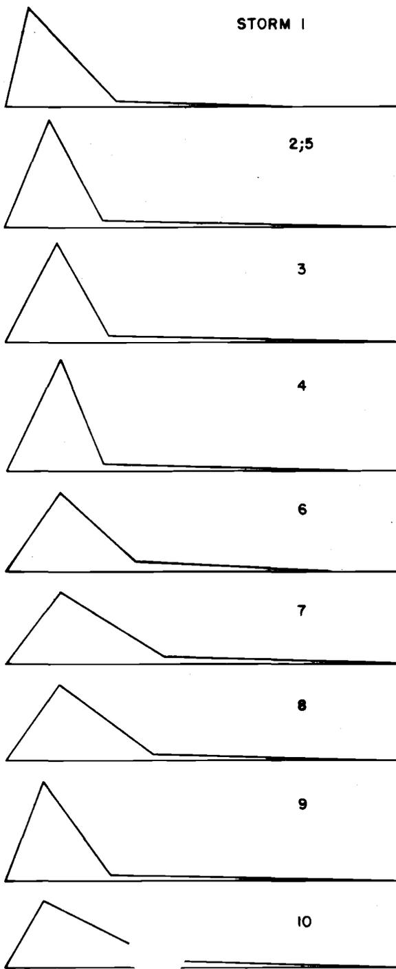
Fig. 5.-- Individual optimal unit hydrographs for the ten storms.
