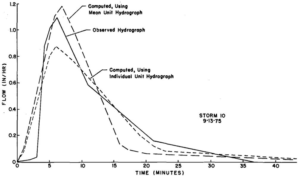
Fig. 7 -- Observed and computed runoff hydrographs for storm of Sept. 13, 1975 (No. 10).
