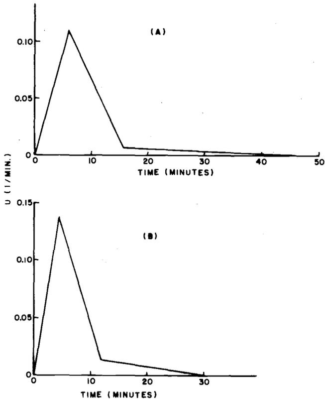
Fig. 4 -- Mean optimal unit hydrographs: (A) based on minimum sum of absolute deviations, (B) based on minimum magnitude of peak difference.
