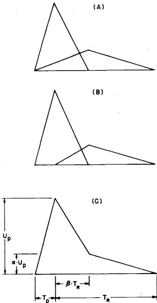
Fig. 3 -- The double triangle unit hydrograph.
