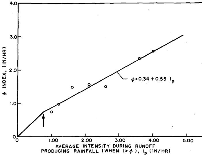
Figure 2. Average loss rate,  $\phi$ -index, vs. average intensity of runoff producing rainfall,  $I_p$ , watershed 76.001.
