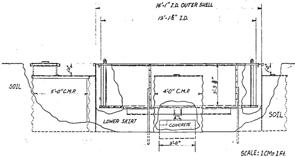
Figure 2. Plan View of Lysimeter, Electronic Transducer, and Access Equipment Wells
