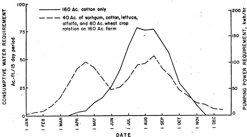
Figure 1. Consumptive water and pumping power requirement for two cropping systems at Mesa, Arizona. Running water level is 300 feet, water application efficiency is 70 percent and pump-power plant energy efficiency is 65 percent.
