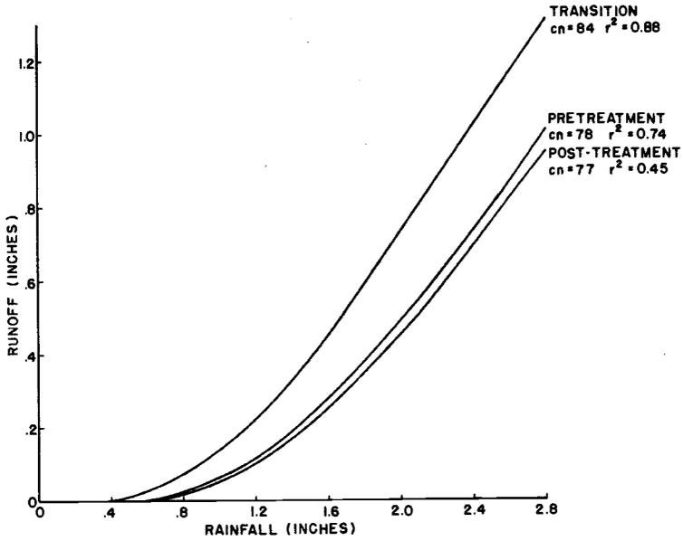
FIGURE 4a. RAINFALL VS. RUNOFF. SCS CURVE NUMBER.
