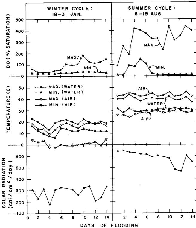
Figure 1. Effect of algal development and related seasonal (winter and summer) influences of temperature and solar radiation on dissolved oxygen concentrations in recharge soil basins flooded with secondary sewage effluent for 14 days.
