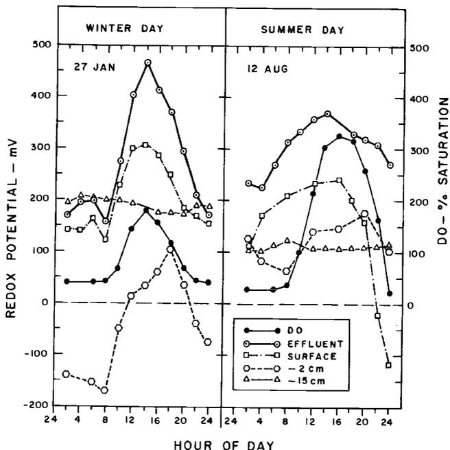
Figure 2. Diurnal fluxes of dissolved oxygen and redox potentials in soil basins flooded with secondary sewage effluent on a selected winter and summer day.
