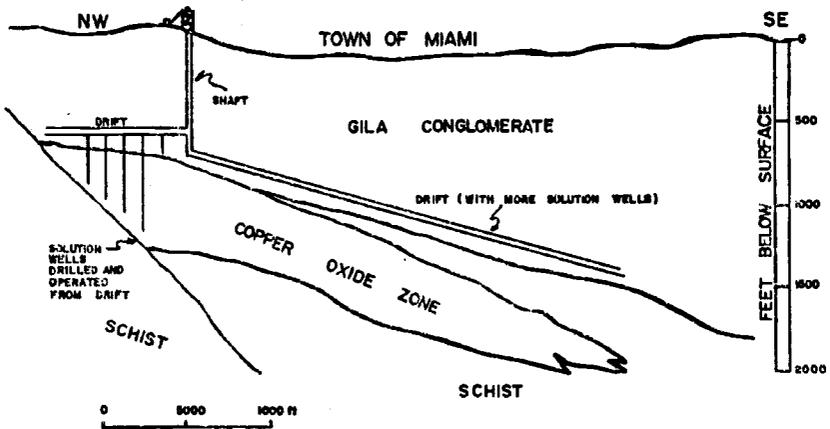
Figure 4: VERTICAL CROSS-SECTION THROUGH VAN DYKE COPPER ORE DEPOSIT. FULL SCALE PRODUCTION BY OCCIDENTAL MINERALS CORPORATION, DENVER, COLORADO CONSISTS OF SINKING A VERTICAL SHAFT OUTSIDE THE TOWN LIMITS AND DRIFTING HORIZONTALLY BELOW THE TOWN AND IMMEDIATELY ABOVE THE ORE BODY. THE ACID INJECTION AND RECOVERY WELLS WILL BE DRILLED AND OPERATED FROM THE UNDERGROUND DRIFTS
