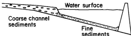
Figure 2.--Idealized cross section of stock tank.
