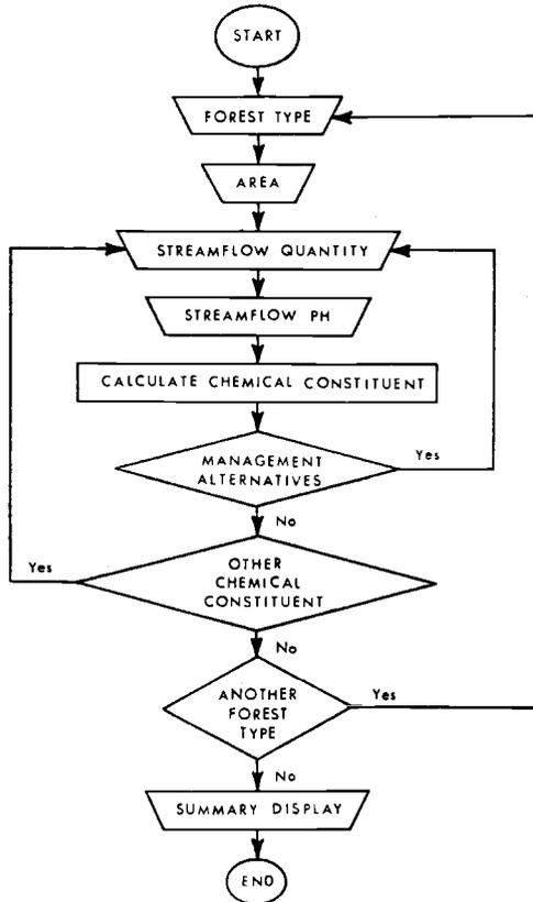
Figure 1 - Flow of activities in executing CHEM to predict dissolved chemical constituents in streamflow.
