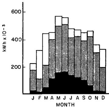
Figure 2a. Solar energy collected in 1980. Clear, crosshatched and shaded areas represent solar energy availability, solar energy available during collector operation and collected thermal energy, respectively.
