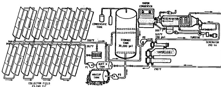
Figure 1. 150-kW Solar-Powered Irrigation Facility Flow Diagram (Duffy et al., 1980)
