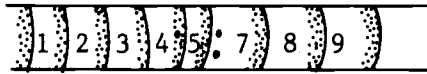
Fig. 10a. The core marking for a combination of a microring and a missing ring. Ring #5 is the microring and Ring #6 is the missing ring.
