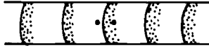
Fig. 9b. What the core marking for a microring looks like when the microring cannot be seen.
